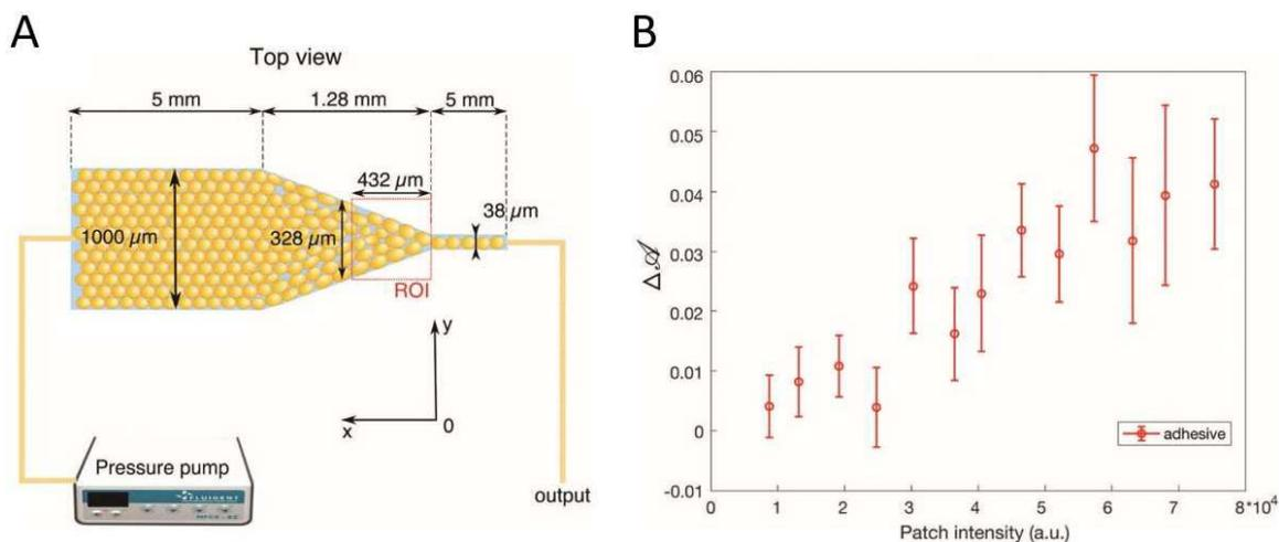
Fig. 16. A. Experimental setup for flowing an oil-in-water emulsion through a microfluidics constriction. B. Shape parameter  $\mathcal{A}$  before and after undergoing a T1 rearrangement as a function of the patch intensity. From [118].
