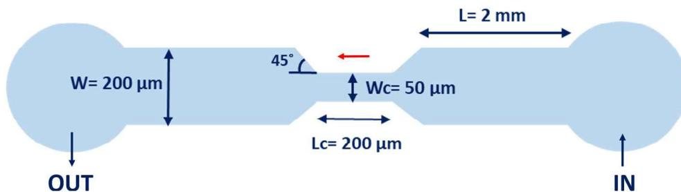
Fig. 25. Sketch of the geometry of choice for the microfluidic aspiration experiments. The height of the channel is  $40 \mu\text{m}$ . The red arrow indicates the direction of the flow. Drawing not to scale.
