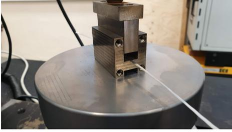
Figure 2.5: Single yarn compression device
