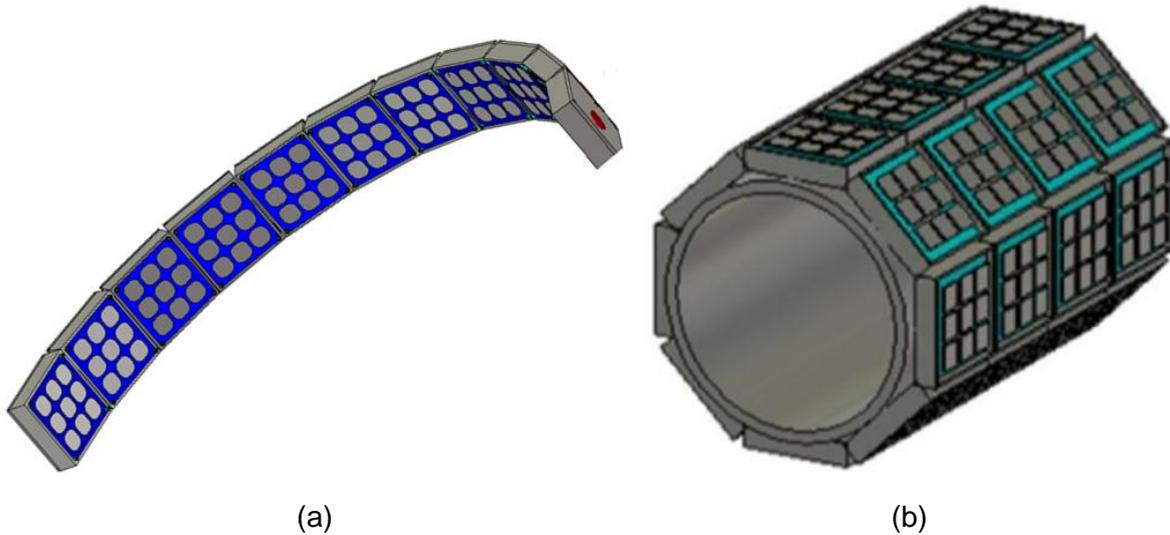
Figure II. 6: Architectures des antennes MARPEM conformes (a) 1D concave (b) 2D convexe.
