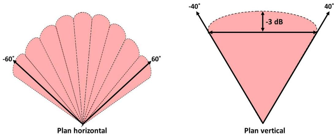
Figure V. 16: Balayage de faisceaux sectoriels.
