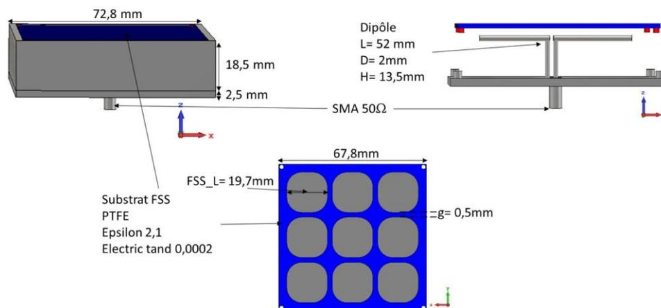
Figure IV. 1: Structure du Pixel large bande.
