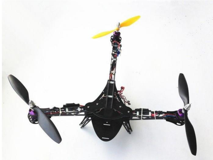
FIGURE 1.4 – Exemple de drone tri-rotor
