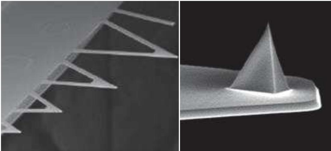
*Figure 26: Cantilevers and tip of a Bruker MSNL AFM probe*
