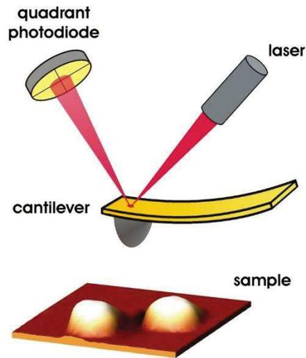
*Figure 25: AFM principle. A laser is reflected at the back of a cantilever equipped with a nanometric tip at its end. By measuring the deflection of the reflected laser beam with a photodiode when the tip is in contact with the sample it is possible to reconstruct its topography at the nanometric scale by scanning a small area.*
