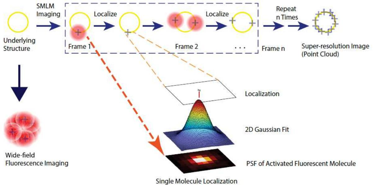
*Figure 36: SMLM principle. A structure of interest is fluorescently labelled. Widefield fluorescence imaging cannot resolve it. By recording  $n$  frames in which only few molecules per frame are emitting fluorescence, it is possible to fit the PSF of single molecules by a 2D gaussian and to precisely determine its position. All localizations are then assembled into a super-resolution image which corresponds to a map of localizations. Illustration from Khater *et al.*, 2020.*
