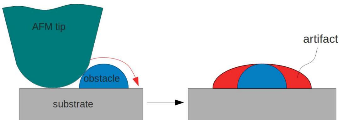
*Figure 27: Tip convolution and resulting artefact (red) in AFM imaging
