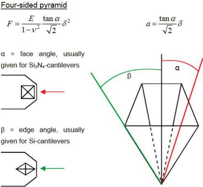
*Figure 29: Equation describing the force between sample and a four-sided pyramidal tip. By fixing the tip geometry it is possible to extract an effective Young Modulus with the force and indentation parameters extracted from QI force curves.*
