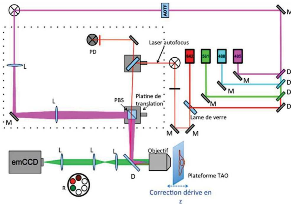
*Figure 38:* Schematic of the setup used for correlative AFM/fluorescence microscopy. M: mirror, D: dichroic mirror, L: lens, R: filter wheel, PD: 4-quadrant photodiode (autofocus), PBS: polarized beam splitter.
