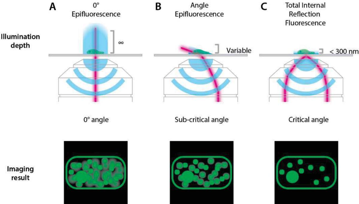
*Figure 32: Epifluorescence, angle epifluorescence (also known as Hilo) and TIRF microscopy illumination scheme and corresponding image illustration of the signal to noise ratio. Adapted from Vangindertael et al., 2018.*
