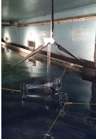
FIGURE 1.11: Experimental model of the semi-submersible from Lacaze [101] tested in the wind-wave tank facility at Marseille-Luminy (France)
