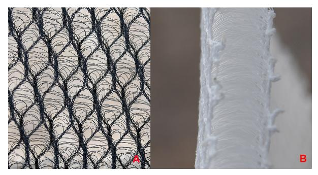
Figure 5. Examples of spacer fabric. A. Frontal view of spacer fabric used in the CloudFisher™ system, showing one outer layer of the fabric (dark) with threads from internal layer (grey) visible within the gaps of the outer layer. B. Cross-sectional view
