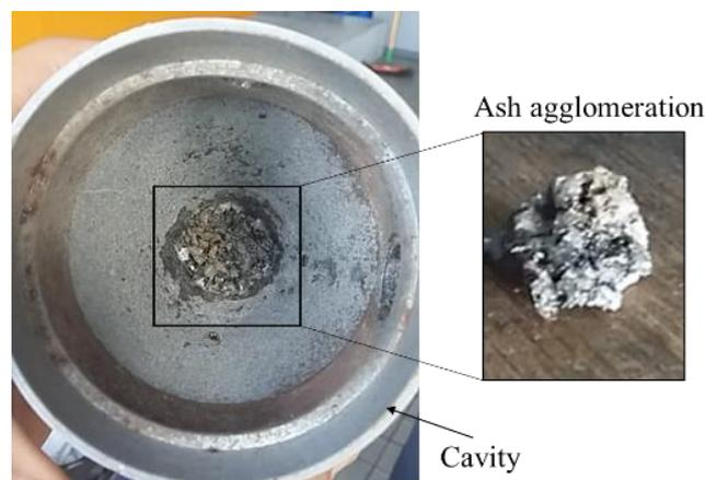
Figure II.40 Top view photography of the solar cavity after Run#2
