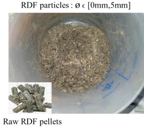
Figure II.35 SRF sample preparation
