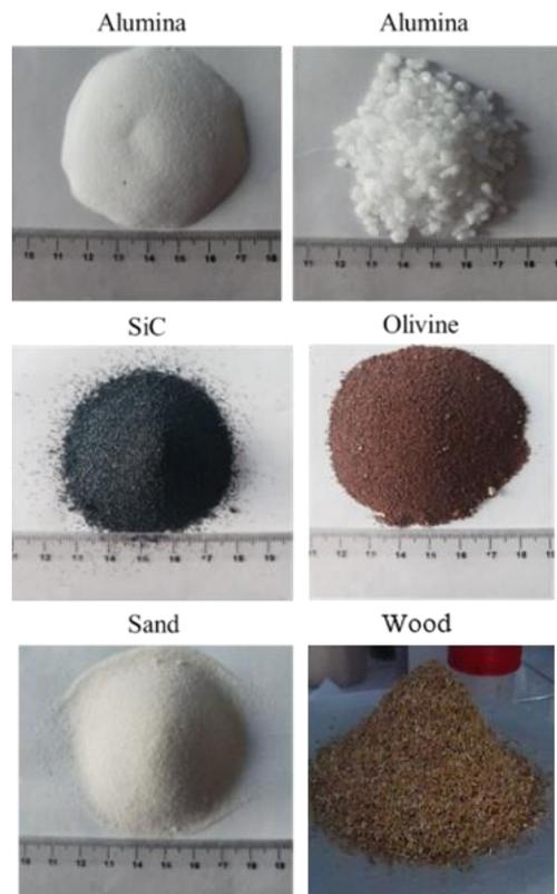
Figure III.2 Studied inert bed and wood biomass particles
