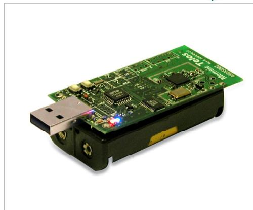
The TelosB platform was developed and published to the research community by UC Berkeley. This platform delivers low power consumption allowing for long battery life as well as fast wakeup from sleep state. The TPR2420 is compatible with the open-source TinyOS distribution.
