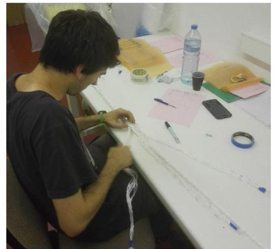
Figure 2-7. Splicing of a 4 ton sub-rop diameter.
