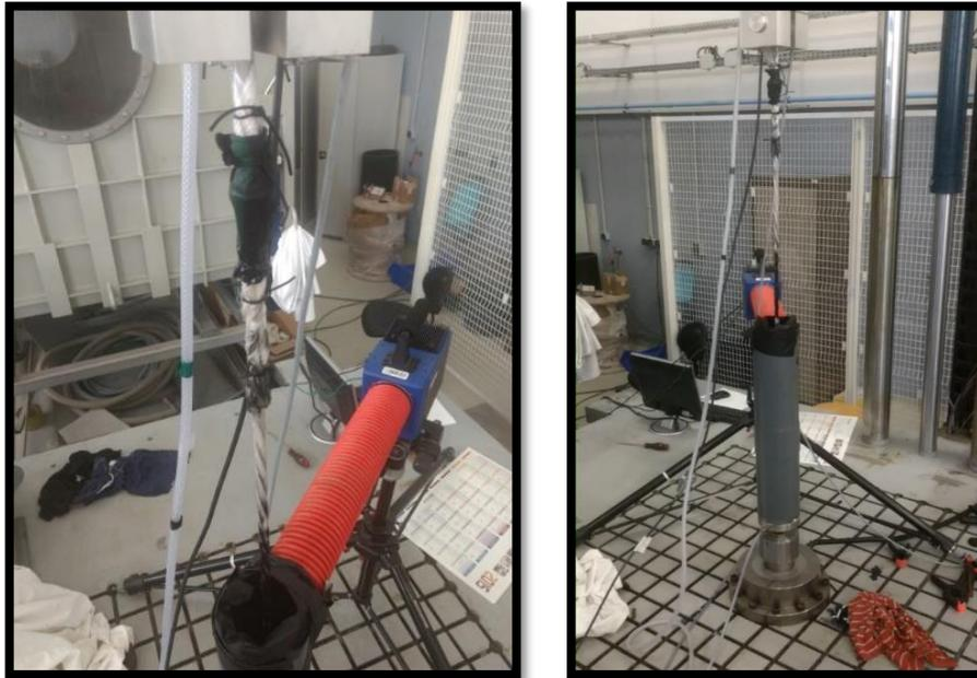
Figure 4-7. 4-tons sub-ropes during a fatigue test.
