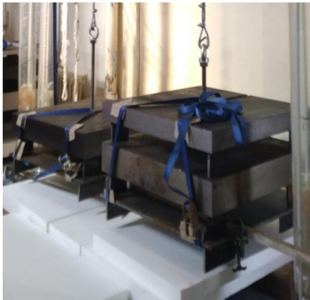
**Figure 7-8. Weight of the long-term creep machine.**
