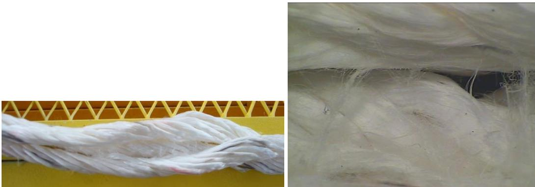
Figure 4-29. Example of internal abrasion in rope sample.
