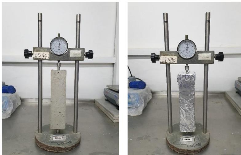
*Figure III.16 The length change readings to determine the total and autogenous shrinkages*
