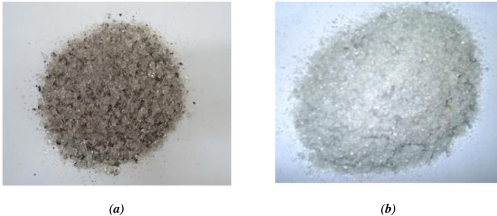
**Figure 1.5 Examples of glass waste used as fine aggregates in concrete**
