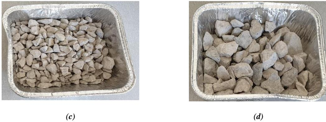
**Figure II.1** Simple observation of (a) natural sand, (b) crushed sand, (c) medium aggregate, and (d) coarse aggregate
