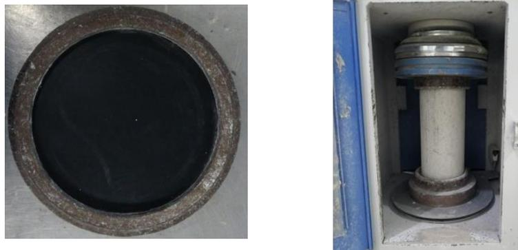
*Figure III.13 Neoprene pad and compressive strength machine*
