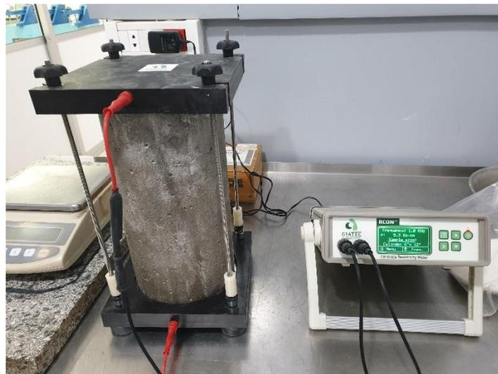
Figure III.19 The apparatus of the resistivity test for concrete specimens
