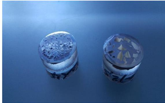
*Figure II.3 Samples preparation of the two types of sand for SEM analysis*
