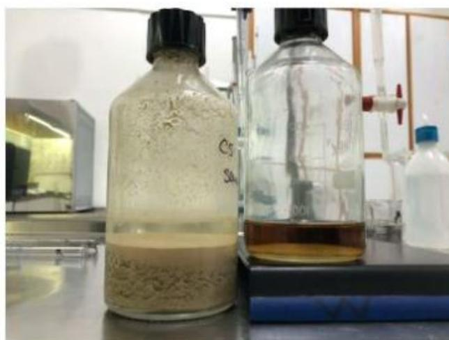
*Figure B.2. Comparison of the crushed sand solution (at the left) to the standard color solution (at the right) to detect organic impurities in crushed sand*
