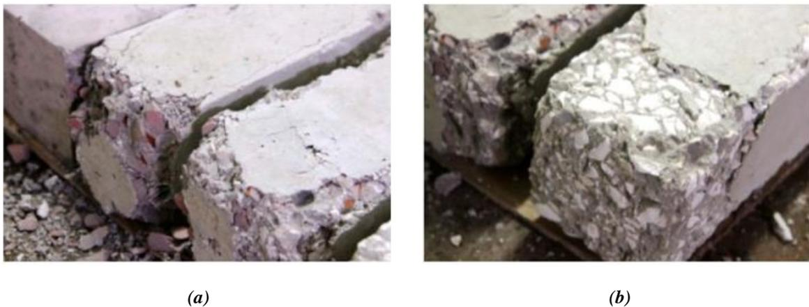
**Figure I.4** The difference of surface spalling, after exposure to a temperature of 1000 °C, between (a) concrete containing crushed bricks and roof tiles aggregates and (b) concrete containing crushed basaltic aggregates (*Miličević et al., 2016*)
