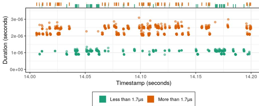
**Figure 10.6.:** Temporal evolution of the MPI\_Recv durations for all the sizes between 1 B and 1 kB during a 0.2 s time window of the non-shuffled experiment. Another temporal pattern can be observed. Durations truncated to  $4\mu\text{s}$  for a better readability.
