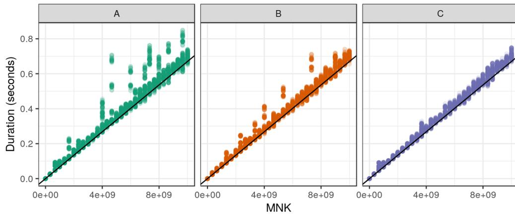
**Figure 10.9.:** Durations of individual `dgemm` calls for CPU 1 of `dahu-5`. Several calls have significantly longer durations than others. Identical black line on the three plots, with slope  $6.7 \times 10^{-11}$ .
