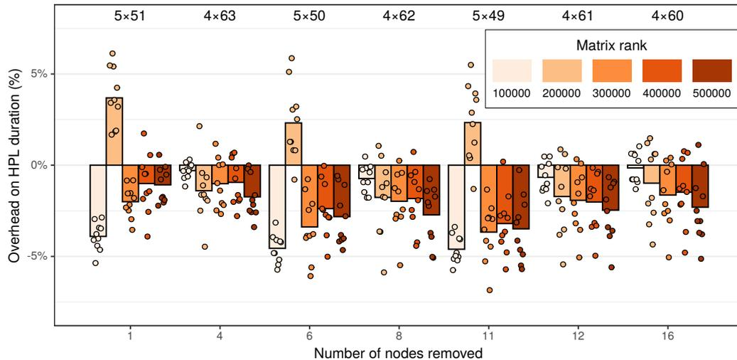
**Figure 7.4.:** Influence of node removal on performance in a stronger heterogeneity scenario (extrapolation of our test cluster when it had a cooling problem on 4 of its nodes). Removing 6 to 12 nodes out of 256 nodes may bring substantial improvement and such optimization would therefore be worth investigating.
