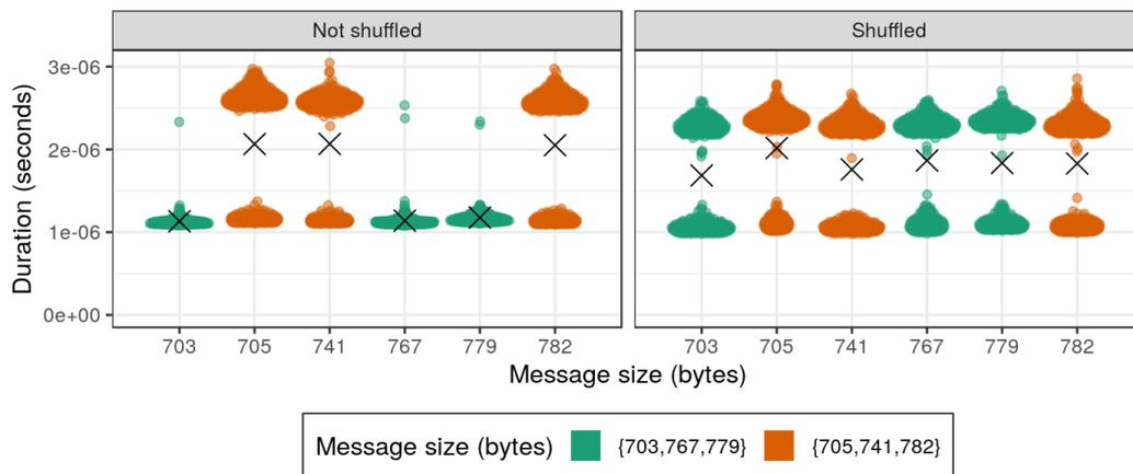
**Figure 10.4.:** Distribution of the `MPI_Recv` durations for six different message sizes between 700 B and 800 B. The durations are not identically distributed in the non-shuffled case. Durations truncated to  $4\mu s$  for a better readability.
