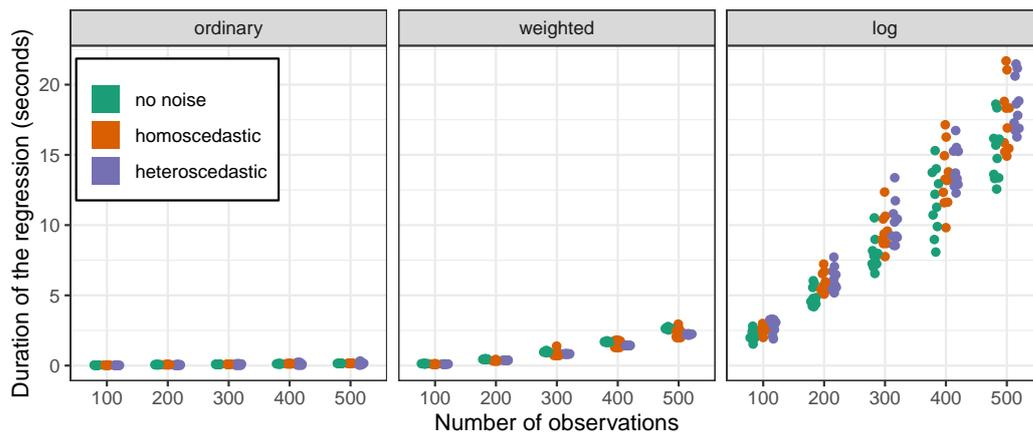
**Figure 5.9.:** Duration of a complete regression with piecewise for different numbers of observations.
