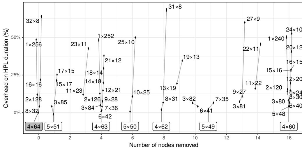
**Figure 7.2.:** Influence of the number of nodes on the performance of HPL. The geometry of the virtual topology is particularly influential, and it appears that  $P \times Q$  configurations with a small P perform significantly better than those with a larger P. Each configuration is summarized through the average overhead over the 10 clusters and error bars represent a 95 % confidence interval.
