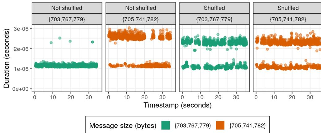
**Figure 10.5.:** Temporal evolution of the MPI\_Recv durations for six different message sizes between 700 B and 800 B. A temporal pattern can be observed. Durations truncated to  $4\mu\text{s}$  for a better readability.
