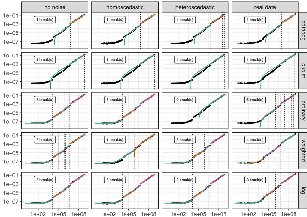
**Figure 5.7.:** Illustrating different piecewise linear regression approaches on different datasets. Only our implementation (pycwise) with the logarithmic objective function works well for all datasets.
