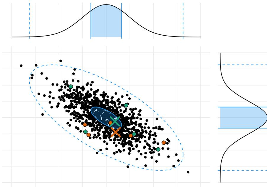
**Figure 11.3.:** Illustrating the proposed test with two sets of five observations ( $r = 5$ ) and a bivariate normal distribution ( $p = 2$ ). The blue dashed lines represent the 99.5% prediction regions for single observations, the blue zones represent the 99.5% prediction regions for the averages of five new observations, represented by crosses.
