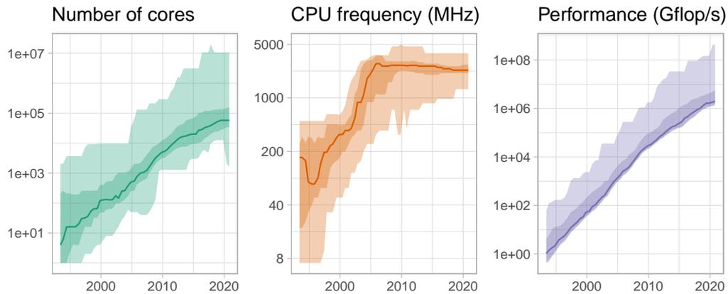
**Figure 1.3.:** Evolution of the Top500 [top500] supercomputers between 1993 and 2020. The line denotes the median, the inner ribbon contains the [10 %, 90 %] interval, the outer ribbon contains all the values. Data compiled by Dan Lenski [Len20] and plotted by ourselves.
