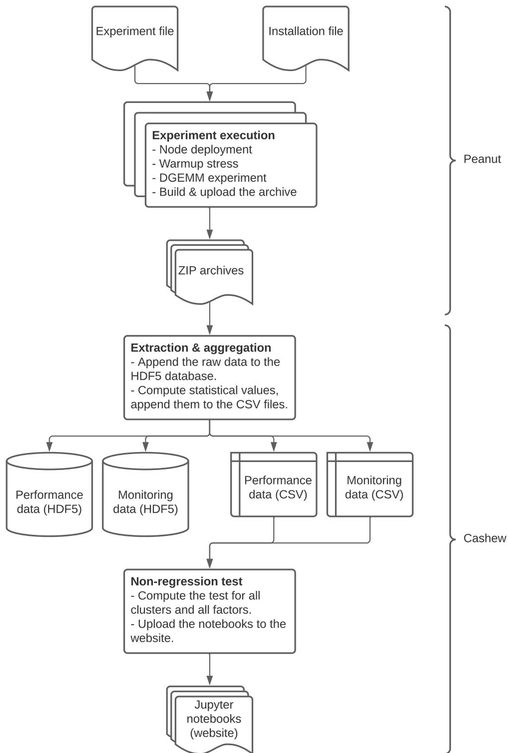
Figure 11.4.: Full workflow implemented by our tests.
