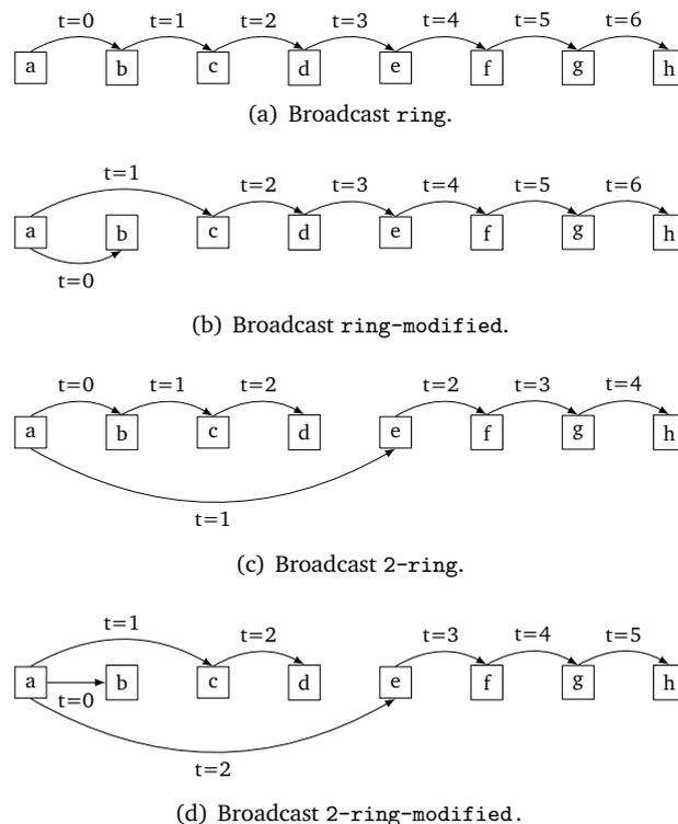
**Figure 3.2.:** Illustration of the four HPL ring-broadcast algorithms.
