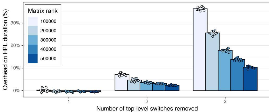
**Figure 7.5.:** Influence of the physical topology on the overall performance. It is possible to remove up to 2 of the top-level switches without significantly hurting performances for large matrices. Beyond this point, communications become the main performance bottleneck.
