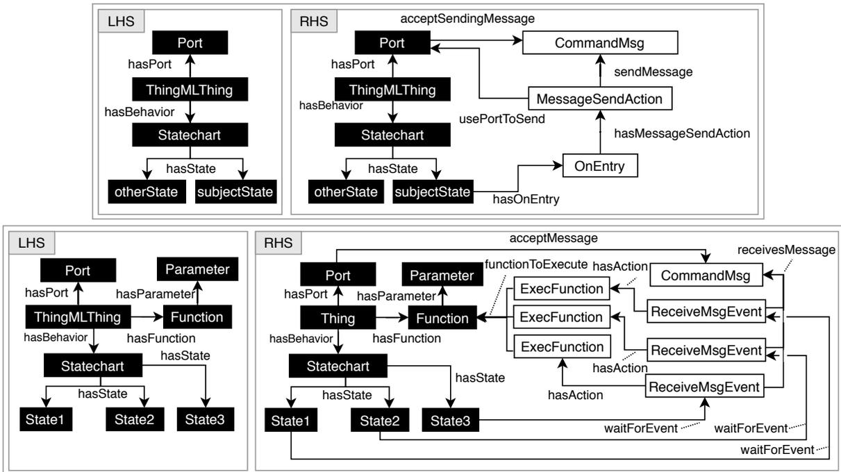
Figure 4.11 – Upper Part for Subject, Lower Part for Object; applying the `trigger:executeFunction` rule GTRs (3) with the subject thing having two states and the object thing having three states; white boxes are added based on the CY-Model.
