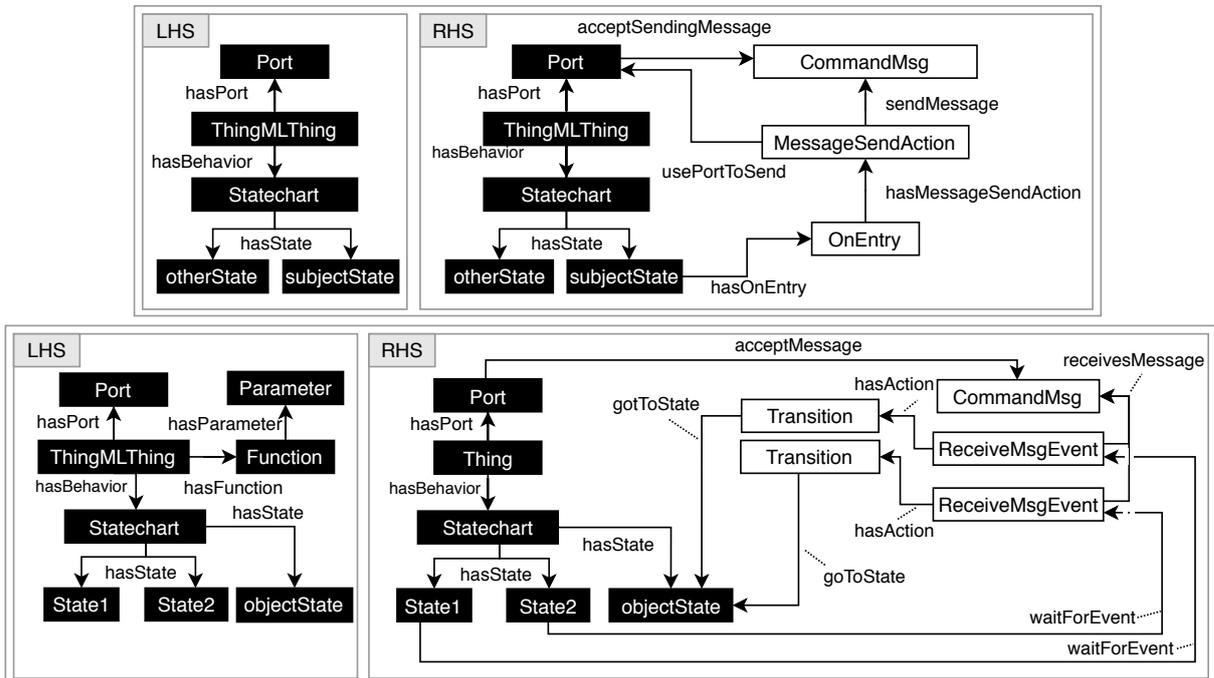
Figure 4.12 – Upper Part for Subject, Lower Part for Object; applying the *trigger:goToState* rule GTRs (4) with the subject thing having two states and the object thing having three states; white boxes are added based on the CY-Model.
