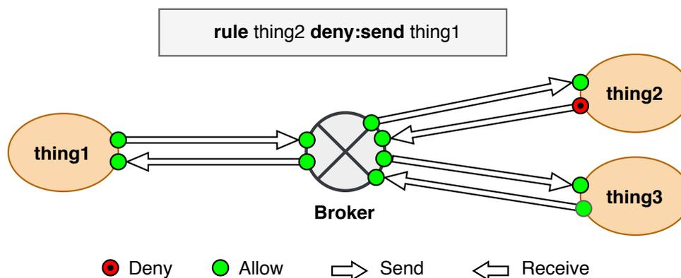
Figure 4.7 – Enforcement at the “on send” checkpoint
