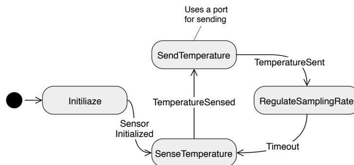
Figure 2.3 – Statechart-based behavior of a temperature sensor
