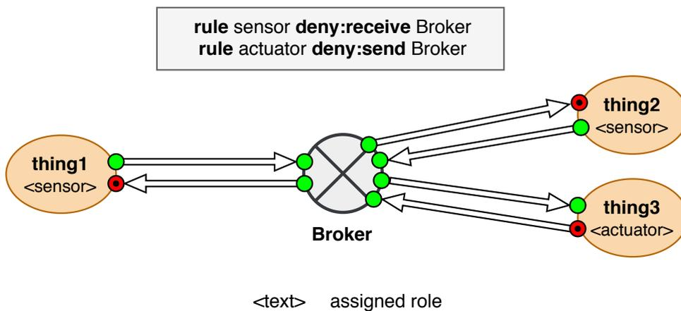
Figure 4.9 – Enforcement of a role-based rule
