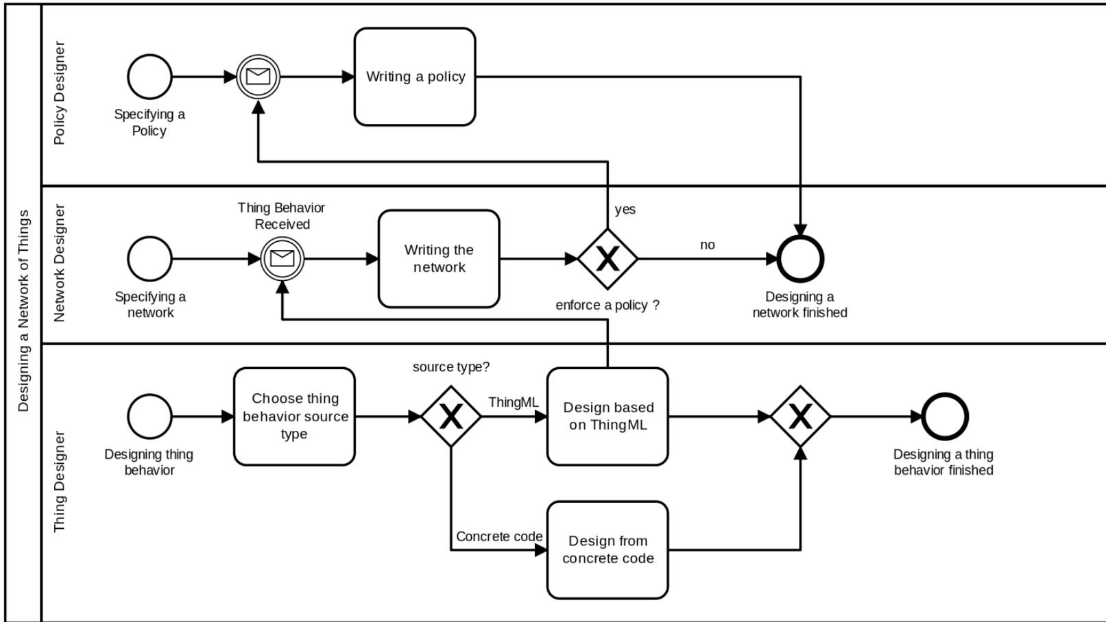
Figure 5.1 – BPMN diagram of the methodology
