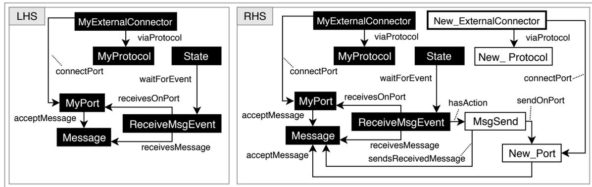
Figure 4.3 – Upper Part (GTR (1)): Adding the communication interface according to the specification of the network. Lower part (GTR (2)): Forwarding an existing binding; white boxes are added based on the CY-Model; the added External Connector box is thicker for readability purpose only.
