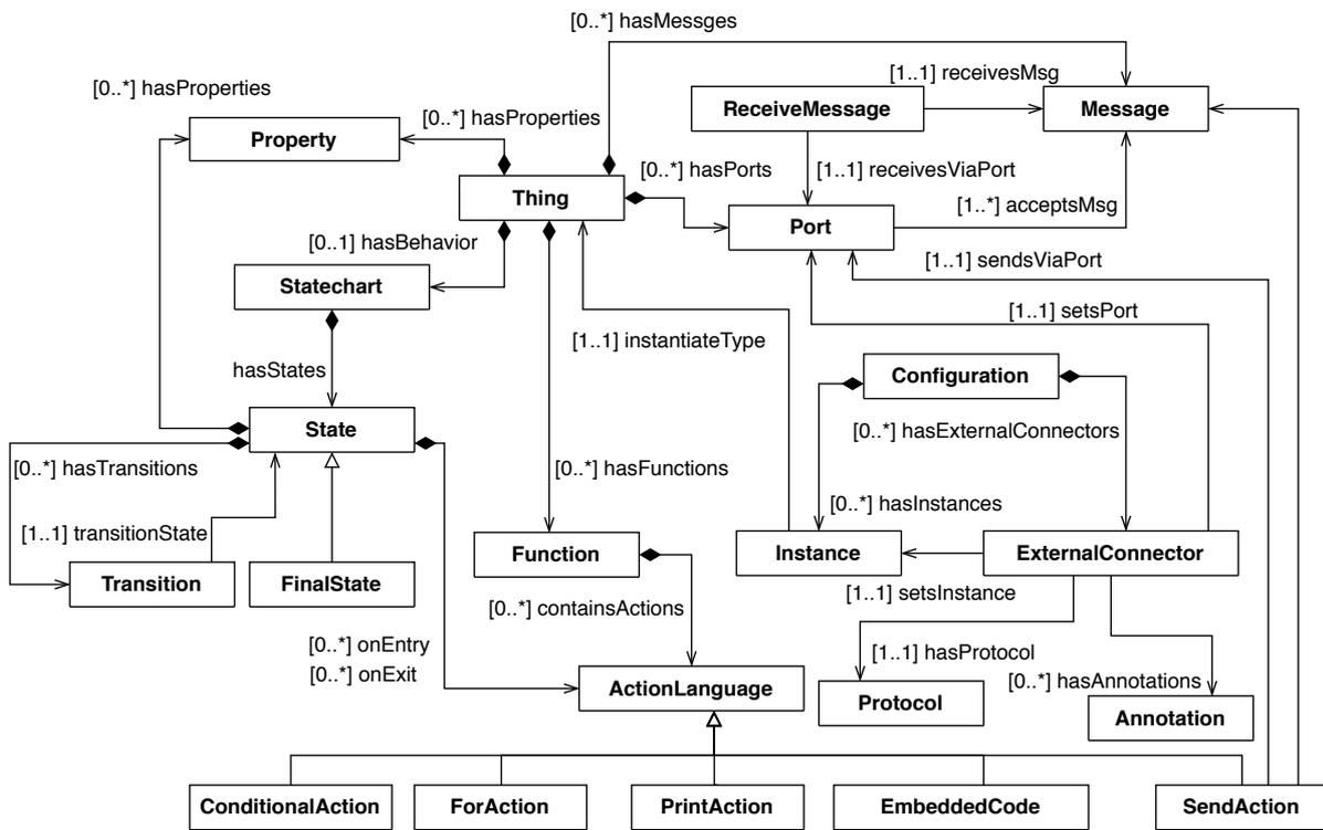
Figure 2.2 – A simplified version of the ThingML metamodel
