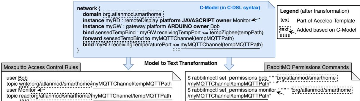
Figure 4.4 – Generation of access control rules for Mosquitto and RabbitMQ using M2TT; same information indicated with same sign; for RabbitMQ syntax, first argument (" ") is for *configure* permission, second for *write* permission and third for *read* permission.
