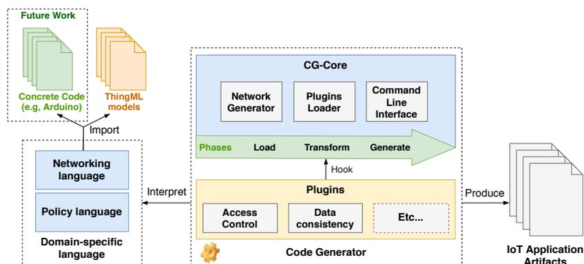
Figure 4.1 – The core components of the code generator
