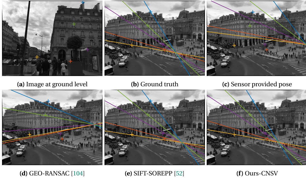
Figure 3.4: Illustration of pose estimation results between a ground level view (a) and an overview camera. The quality may be assessed visually based on the position of the manually defined control points with respect to their epipolar lines and based on the location of the epipole.
