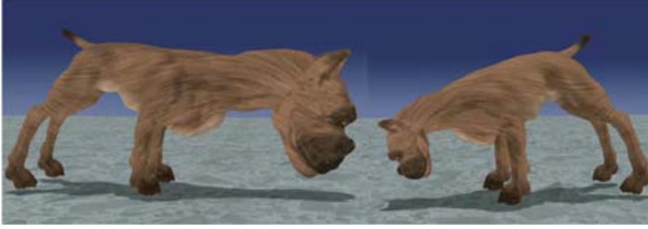
Figure 2.2 – Large rotational deformations yields to inflation artifacts when not using Co-rotational Finite Element Method [MG04].
