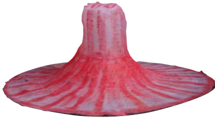
Figure 5.3 – Photogrammetry reconstruction of the real suction cup.
