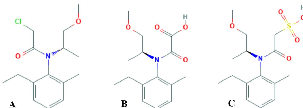
**Figure 4** A Metolachlor (C<sub>15</sub>H<sub>22</sub>ClNO<sub>2</sub>) with its two main degradation products: B MOA (C<sub>15</sub>H<sub>21</sub>NO<sub>4</sub>) and C MESA (C<sub>15</sub>H<sub>23</sub>NO<sub>5</sub>S). Source: <https://pubchem.ncbi.nlm.nih.gov>.
