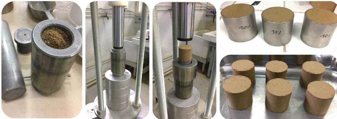
**Figure 2.16** – **From left to right:** (i) compaction device with soil uncompact, (ii) and (iii) compaction press and compacted soil sample, (iv) several compacted soil samples with and without cylindrical molds.
