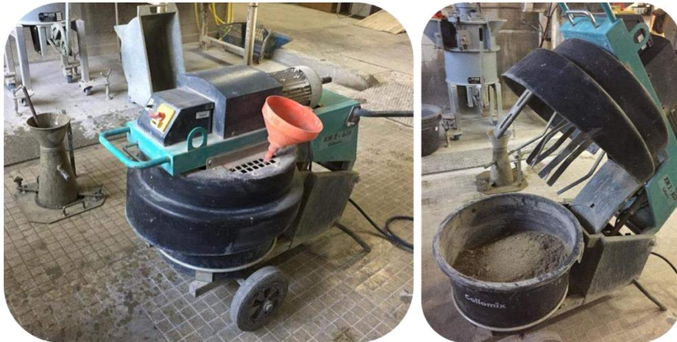
**Figure 2.10** – Concrete mixer “Collomix 25 L” used to fabricate the concretes.
