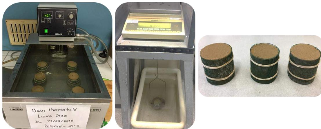
**Figure 2.27 – From left to right: (i)** heated bath employed for keeping water at 40°C for volume expansion tests, **(ii)** device of Archimedes' principle, and **(iii)** example of a series of samples used for volume expansion tests according to the French Standard NF P 94-100.
