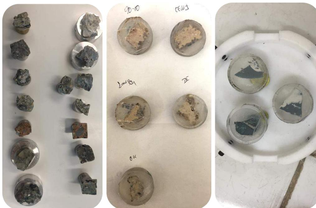
**Figure 2.20** – Examples of samples used for microstructural observations. From left to right: (i) concrete fracture sections, (ii) soil treated samples mounted in resin, and (iii) Mo-spiked binders mounted in resin.
