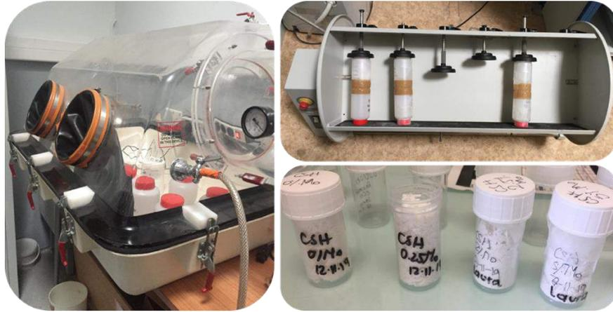
**Figure 2.19** – At left, glovebox under nitrogen employed for the synthesis of C-S-H with Mo. At top right, end-over-end tumbler used to shake solutions. At bottom right, synthetic C-S-H samples obtained after filtration.
