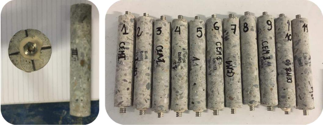
Figure 2.12 – One series of cylinder samples of 150 mm height and 29 mm ± 1 mm diameter with stainless steel nuts positioned at the extremities.
