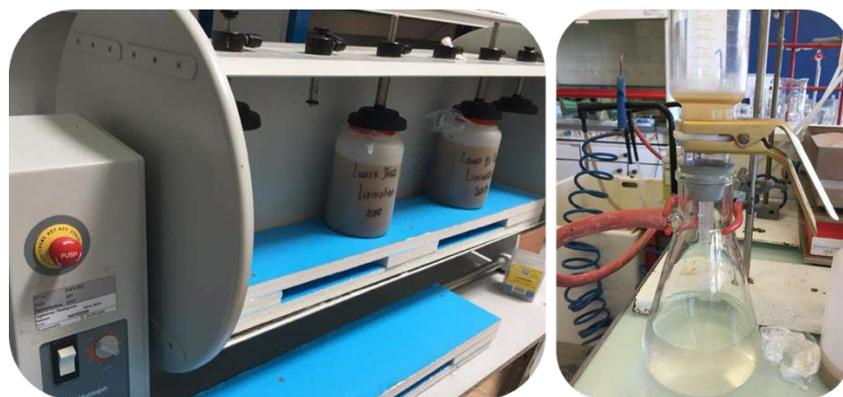
**Figure 2.21** – At left, end-over-end tumbler for leaching tests. At right, vacuum device used for filtration.
