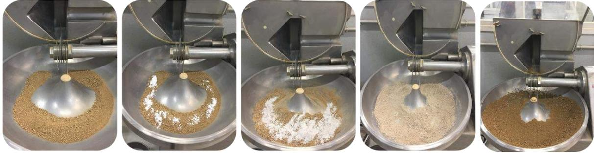
**Figure 2.15** – Preparation of soil samples. **From left to right:** (i) dry soil with particle size below 5 mm, (ii) addition of 1.8 wt% gypsum, (iii) addition of 10 wt% binder, (iv) dry mixture for homogenization, and (v) addition of water for mixture and future compaction.
