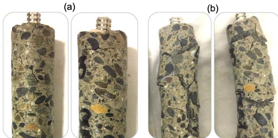
**Figure 3.24** – Pictures of some samples of the C-I concrete (a) at 70 days of tests showing the presence of cracks, and (b) after one year of supplementary submersion showing the decohesion of the samples.
