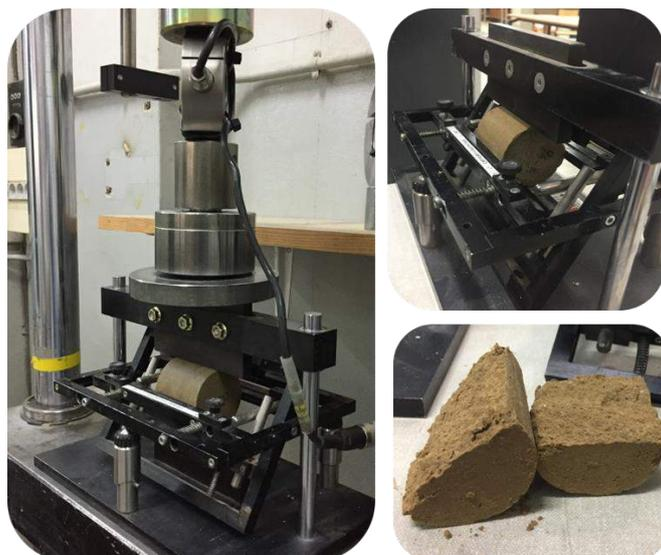
**Figure 2.28** – Device used for splitting tests according to European Standard NF EN 13286-42. **At bottom right:** example of the fracture of a soil sample after splitting test.
