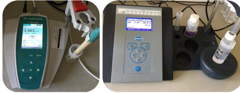
Figure 2.22 – At left, device for conductivity measures. At right, device for pH measures.
