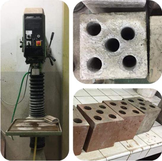
Figure 2.11 – At left, core drill FLOTT type M5 S/N 320201TR used to core the cylinder samples. At right, concrete cubes.
