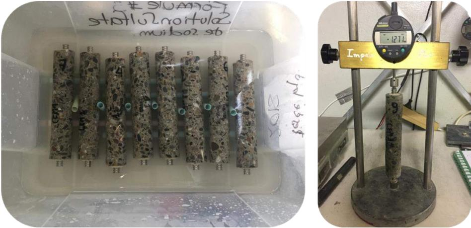
Figure 2.25 – At left, example of a series of samples submerged in the sulfate solution. At right, extensometer device used to measure length variations.
