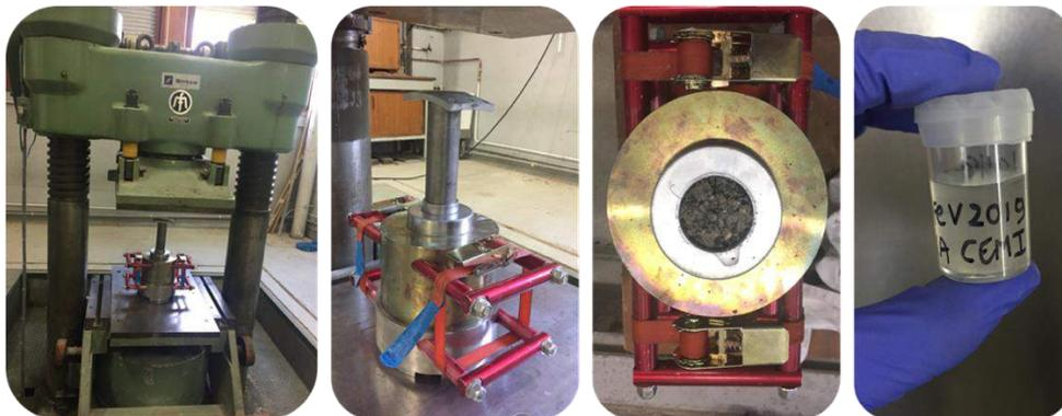
**Figure 2.26** – High-pressure device for squeezing tests. At right, example of solution extracted from C-I concrete after external sulfate attack.
