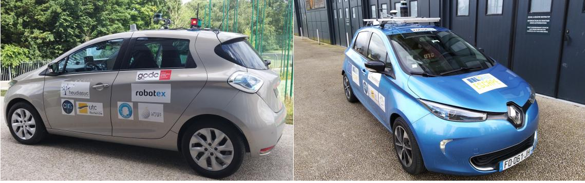
Figure 3.2.: The two vehicles used to obtain experimental data. The gray vehicle (left) is a first generation Renault ZOE ZE which was modified to enable autonomous operation, the blue vehicle is a more recent Renault ZOE ZE which has not been modified for autonomous control.
