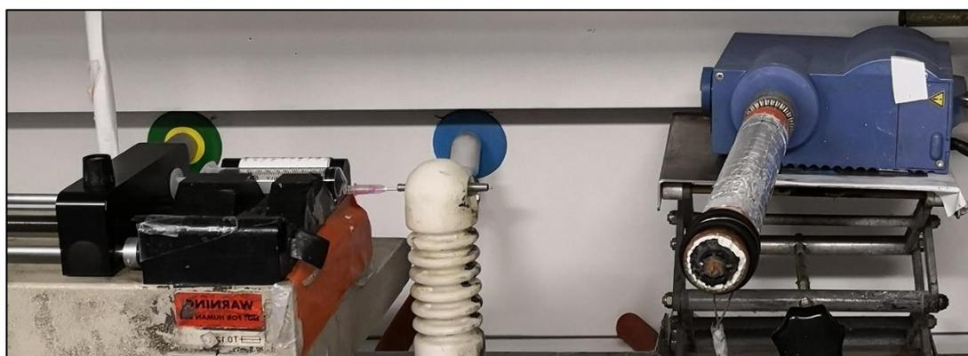
**Figure A.1 - Overview of the base electrospinning setup, without box.**
