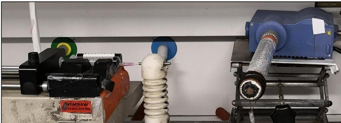
**Figure 2.5 – Overview of a PAN electrospinning setup**
