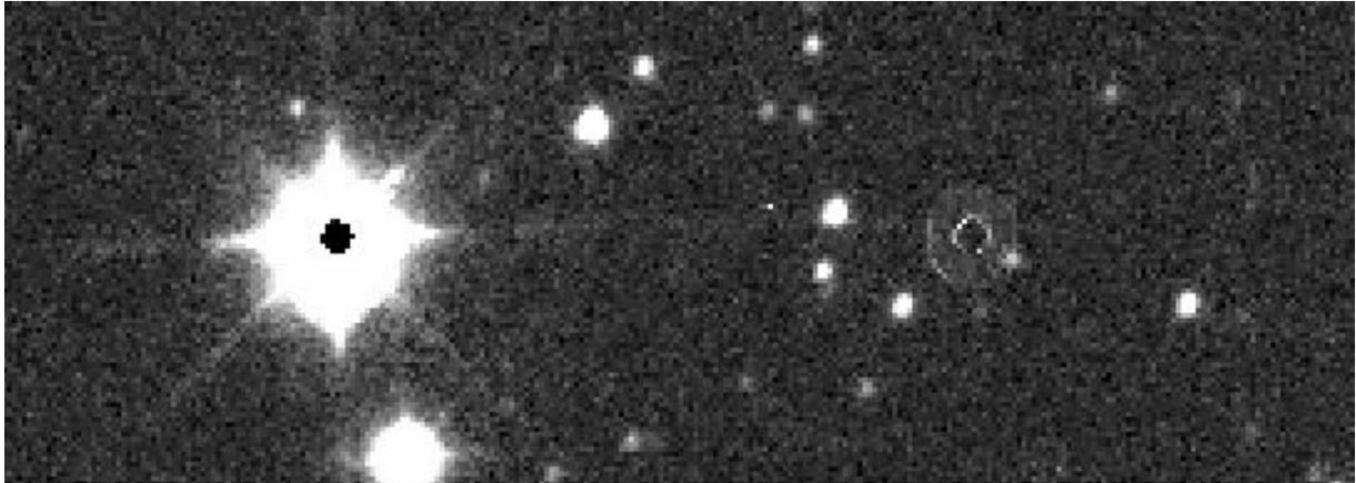
Figure 5.4: Example of a crosstalk pattern between channels in a WFCAM image.
