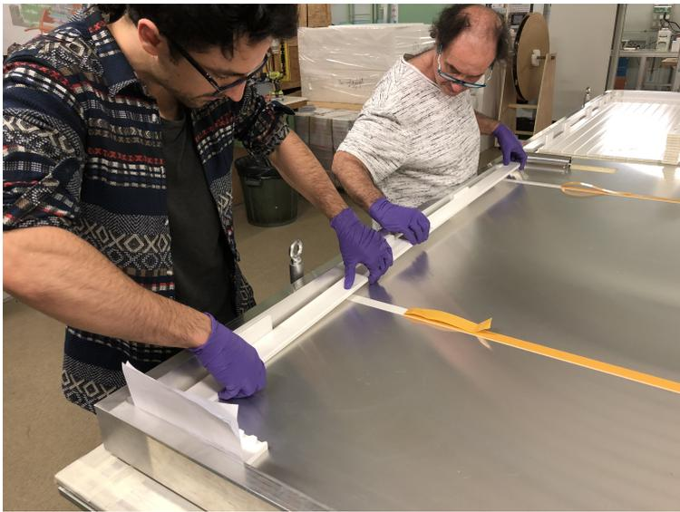
Figure 5.7: Picture of the installation of a scintillator bar inside the aluminum frame. Beforehand, double-sided adhesive stripes are laid out on top of the composite panels two on each side of the module. The protection on the other side of the adhesive stripes are removed as the scintillator bars are installed in the frames.
