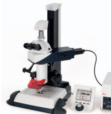
Figure 7. The fluorescence microscope Source: Supplier 2.1 official website
