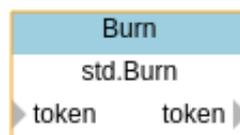
**Figure 6.3:** Burn actor. It receives messages through the input token port in the left, process it, and send it unchanged through the output token port in the right.
