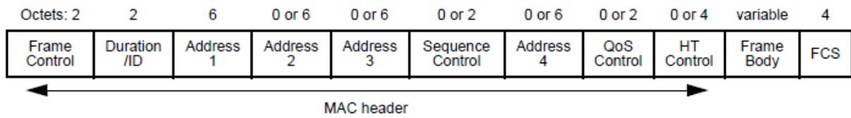
Figure IV-8 : Structure MPDU [46] [136]
