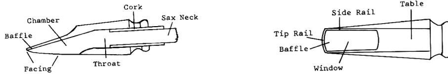
FIGURE 1.4: Side and below schematic views of a saxophone mouthpiece, adapted from [Tea63].
