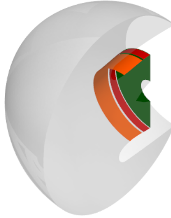
Figure 3.5: 3D view of the intake CAA mesh, which depicts the Inlet surface (orange part in the center of the figure), the Forward Fan Case surface (red part in the center of the figure close to the fan plane), and the excitation plane (green part at the background of the figure)
