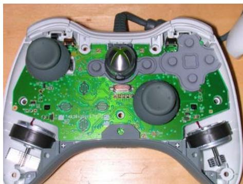
Figure 2-3 – Videogame controller with force feedback motors
