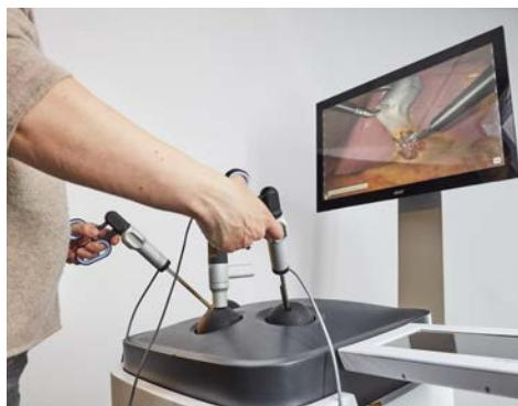
Figure 2-10 – *Lapsim®*: Laparoscopy simulator
