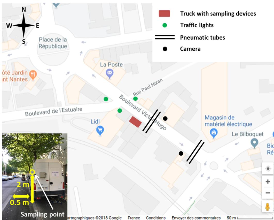
Fig. 1. Diagram of the traffic site used for the measurements.
