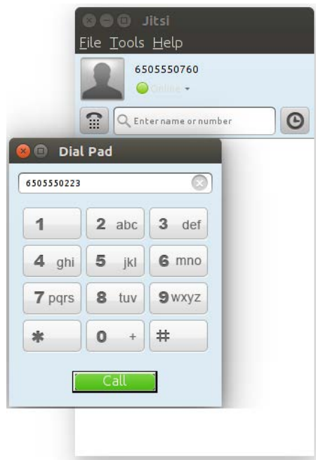
Figure 6 – A connected Jitsi client to the "example.com" base trying to call the client with the SIP number 6505550223.
