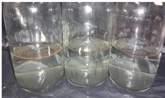
Figure 6.3. Thin layer of red coloured \text{Se}(0) particles on the media in the serum batch bottles with 14.3 \text{ mg.L}^{-1} of selenate, methane in the head space at 2 bars and 5 mL MLG sediment in artificial sea water media.
