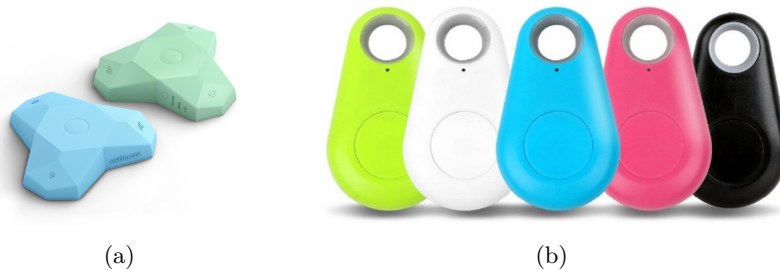
Figure 13: Bluetooth beacons (a) and tags (b)
