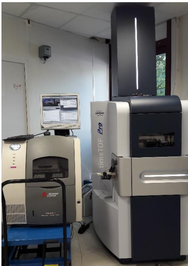
Figure 2.8 : Capillary electrophoresis-Mass spectrometry coupling with a sheathless interface.
