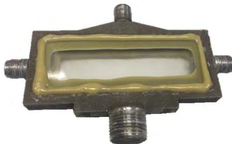
*Figure A 2: Experimental 3D-printed cell after post treatment and with glued microscope slides*
