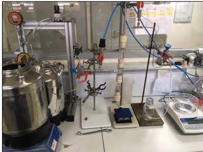
Figure 19: Experimental design of filtration unit A (schematic at the top and picture at the bottom): Filtration in dead-end filtration and outside-in mode under constant pressure and backwash under constant pressure. Experimental pilot equipped with a temperature, pressure and mass recorder.
