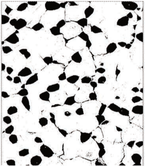
Figure A18.1 Binary images of the microstructure of Ti-18 on transverse section: (a) low-magnification, estimation of surface fraction of globular \alpha_p ; (b) high-magnification image, estimation of surface fraction of acicular \alpha_s ; (c) Zone taken from \beta matrix for image b.
