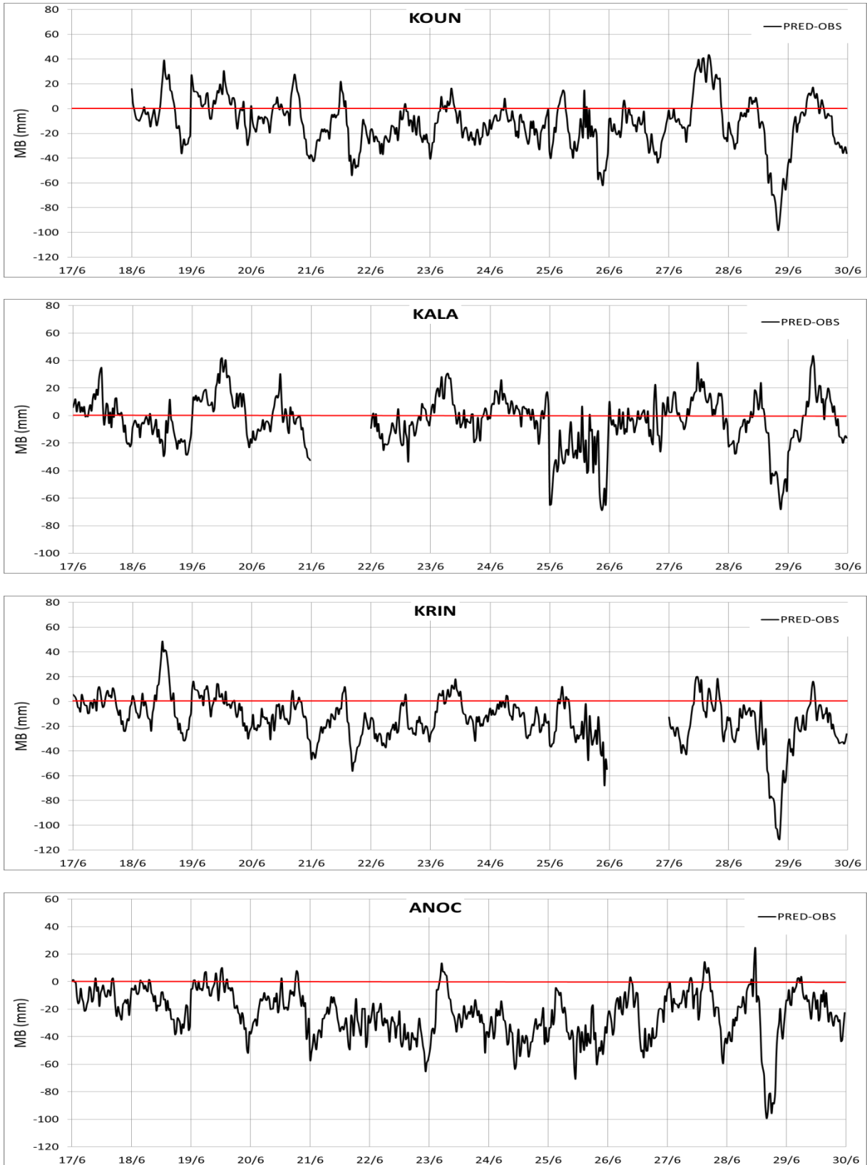
Figure A-20. Bias plots of predicted (WRF MOD5 ASTER) minus observed (GNSS) ZTD at stations KOUN, KALA, KRIN and ANOC.
