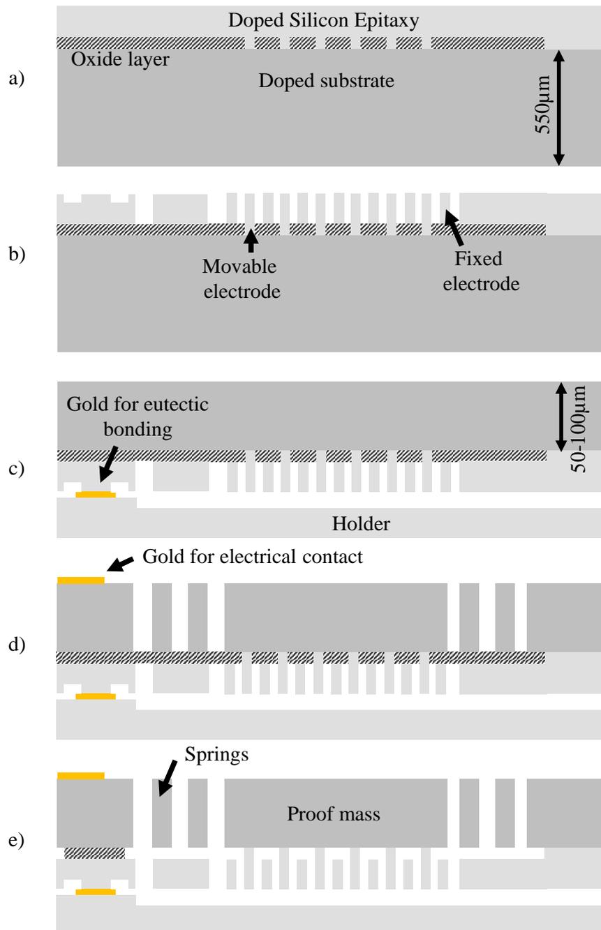
**Figure 2.1:** Schematic view of the fabrication process.
