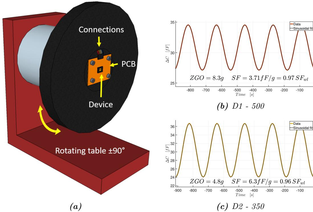
**Figure 4.8:** (a) 3D model of the  $\pm 1g$  test. The device is placed at the center of the rotating table which spins by  $\pm 90$  degrees in order to generate a sinusoidal acceleration of  $\pm 1g$ . (b-c) Scale factor and ZGO evaluation for devices D1-500 and D2-350. The actuation voltage ( $V_m$ ) is set at 1V. The rotating table spins at 2 dps leading to a sinusoidal acceleration of 5.5 mHz. A 4th order 200 mHz LIA filter is used to filter the signal.
