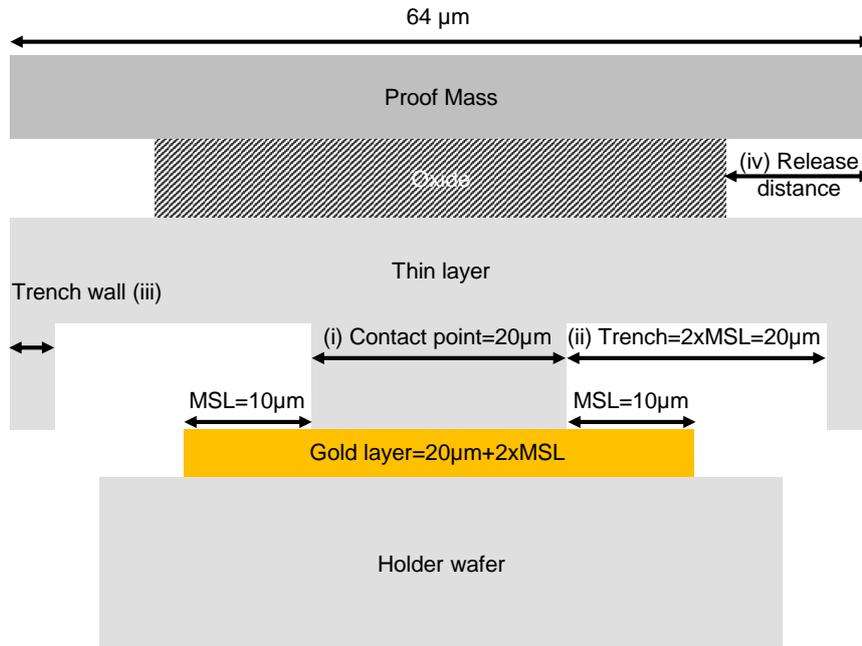
**Figure 2.3:** Cross section of an anchor point: the thin layer is partially etched in order to form a trench around the contact point. The potential misalignment between the holder wafer and the device wafer has to take into account, this leads to an increase in the trench size.
