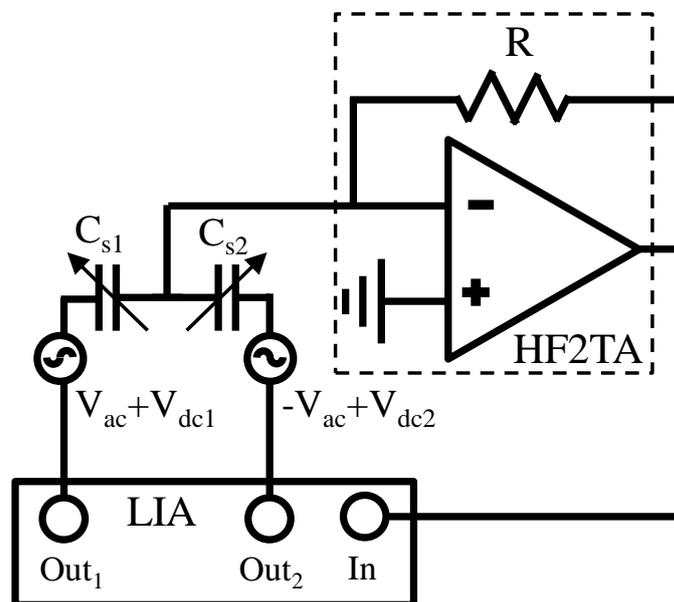
**Figure 4.4:** Schematic of the readout scheme adopted for wafer-level tests: fixed electrodes are polarized with two AC signals of opposite phase, generated by the lock-in amplifier. The current signal is converted into voltage by a dedicated trans-impedance amplifier and demodulated with the LIA. The mass motion is obtained by superposing an actuation voltage to the AC signal.
