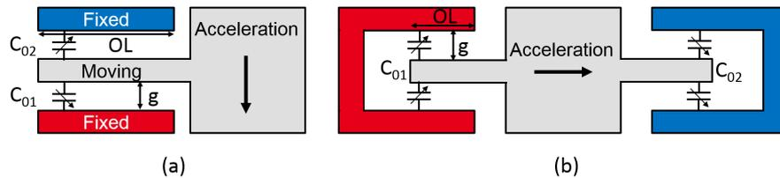
**Figure 2.7:** Scheme of the two main capacitive detection techniques: (a) in gap variation the moving electrodes moves perpendicularly to two fixed electrodes inducing a differential capacitive change, (b) in surface variation the moving electrodes slide parallel to fixed electrodes causing a change in the overlapping area. The two sensing capacitors are referred as  $C_{01}$  and  $C_{02}$ , the gap as  $g$  and the overlap between the two parallel plates as  $OL$ .
