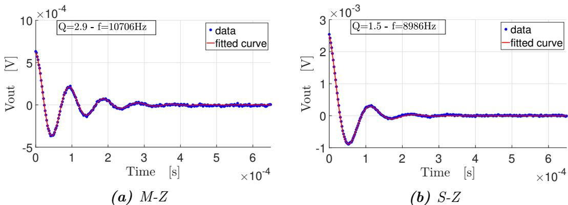
**Figure 5.5:** Ring-down measurement for devices M-Z and S-Z.
