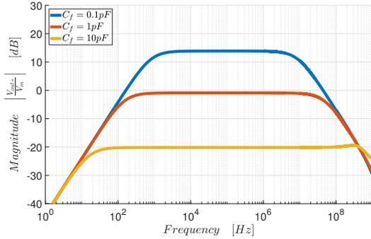
(a) Sweep of feedback capacitance value. The value of the feedback capacitor is swept from 0.1pF to 10pF. Both the gain of the stage and its closed-loop pole shift with the capacitor values.
