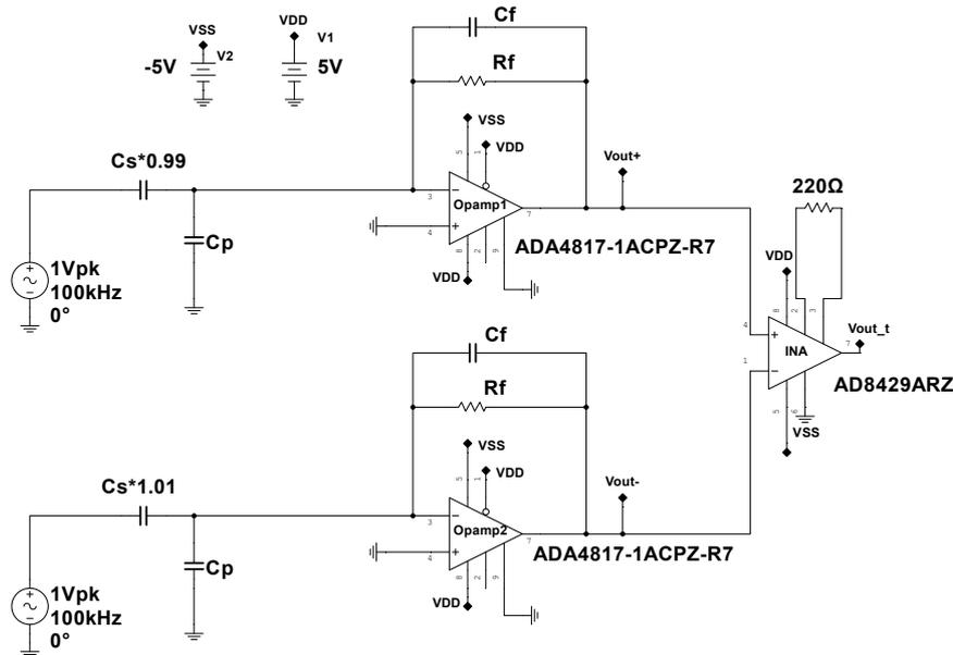
**Figure 3.8:** Schematic of the complete circuit architecture used for software simulations and real PCB implementation.
