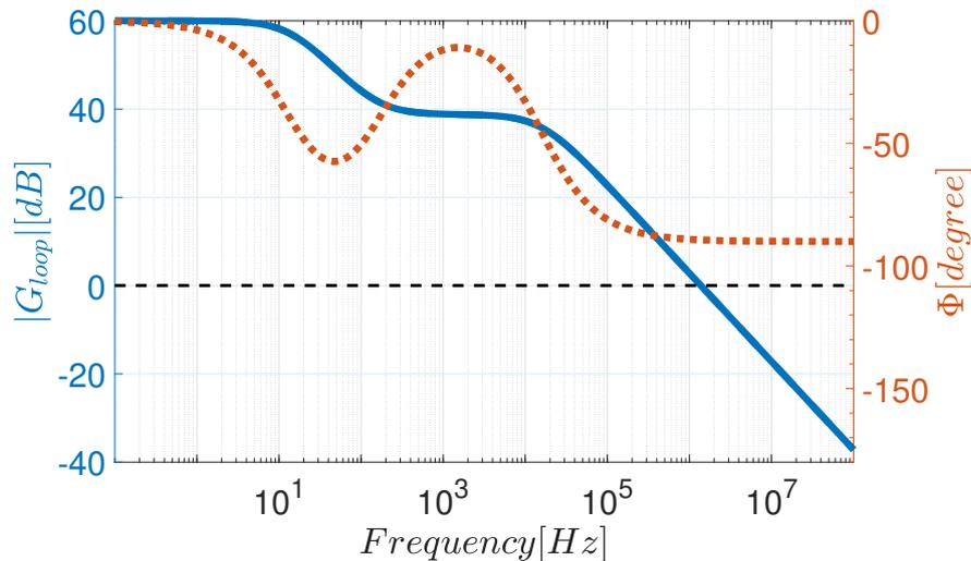
**Figure 3.7:** Bode plot of the circuit  $G_{loop}$ . The phase shift for  $G_{loop} = 1$  is equal to  $90^\circ$  ensuring circuit stability. The singularities of the feedback path cancel each other out and are well below the internal pole of the amplifier.
