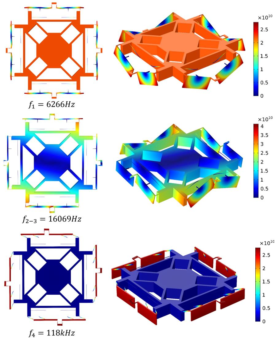
**Figure 2.24:** Different view-points of the modal analysis results for the M-Z device. The desired mode matches analytical prediction within a few percent. The tilting modes are more than a factor two higher than the principal mode thanks to the anti-tilt system. Undesired modes related to the rigid arms are found at 118kHz.
