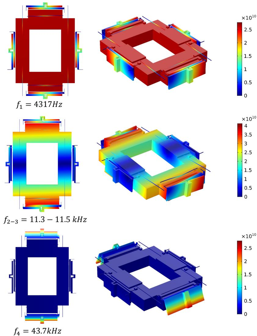
**Figure 2.25:** Modal analysis results for the S-Z device. Again, the mode of interest mode is in line with analytical prediction. The tilt mode frequency changes from 3.8kHz of previous structure to 11.3kHz. The two tilting modes are matched by tuning the width of the central springs, compensating the asymmetry of the structure. High frequency modes related to the rigid arms are a factor ten higher than the desired mode.
