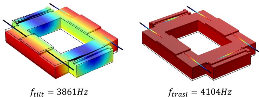
**Figure 2.18:** Mass suspended by flexural springs. Tilting mode is close to desired out-of-plane mode or even at lower frequency. Normal flexural springs allow pure translational movement, but do not impede the tilting of the structure. The problem is worsen by the misalignment between the center of mass and the springs plane.
