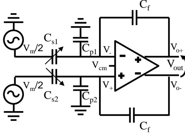
**Figure 3.5:** Schematic view of a fully differential charge amplifier. The voltage generator has been split in two identical sources of halved amplitude. The circuit is considered symmetric exception made for the parasitic capacitance.
