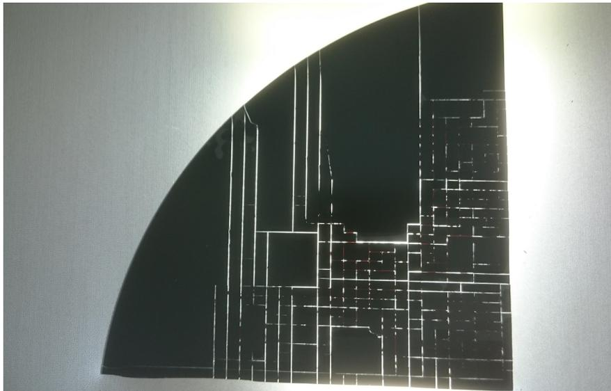
**Figure 4.7:** Image of a quarter of wafer after the dicing procedure. In some areas the separation of the dices was not completed after the laser cut. In those cases, it was necessary to complete the dicing with a mechanical tip.
