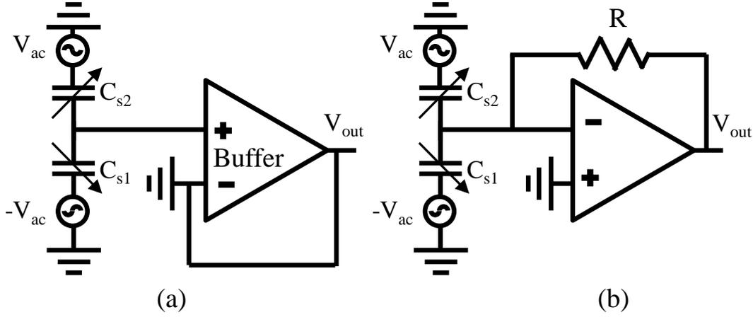
**Figure 3.1:** Schematic view of of: (a) the voltage readout, (b) and current readout for capacitive detection. In voltage readout, the output of the half-bridge is connected to high-impedance node. The voltage change due to the bridge unbalance is reported at the output. In current readout, the bridge output is connected to a low-impedance node. This time the voltage is kept at virtual ground and the current flows into the feedback path of the current to voltage circuit.
