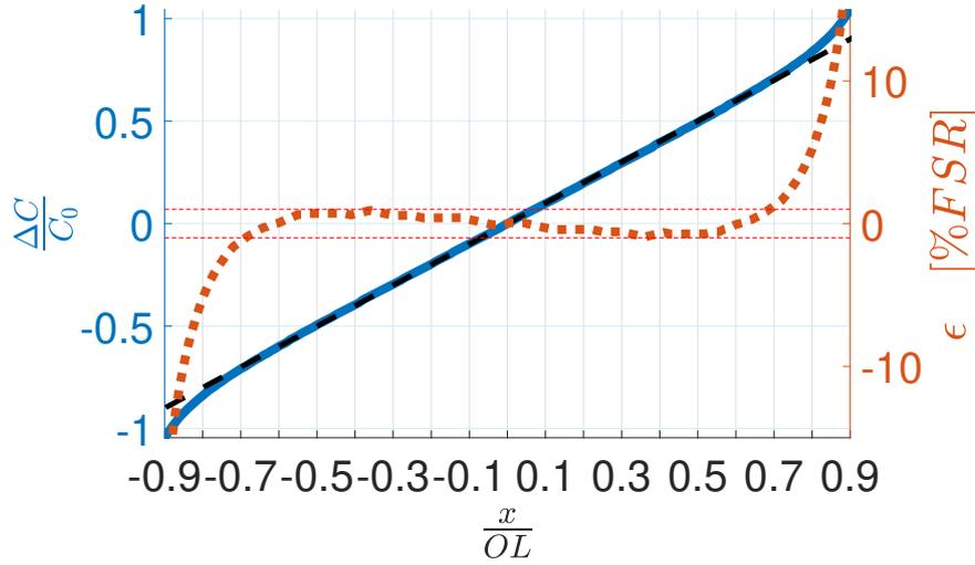
**Figure 2.23:** Plot of the relative capacitive variation and related linearity error with respect to the displacement of the moving comb normalized to the initial overlap for  $z$ -axis detection system at 500nm gap. Nonlinearity greater than 1% occurs at 70% of the relative displacement due to the stray capacitance between the grid and the proof mass. The FSR is evaluated at the point of 1% nonlinearity.
