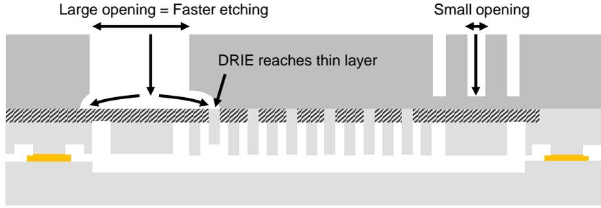
**Figure 2.5:** Schematic cross section of the device during etching of the thick layer. While small opening are being opened, the plasma beam has already reached the stop layer and starts to etch the surrounding silicon affecting some of the thin layer structures.
