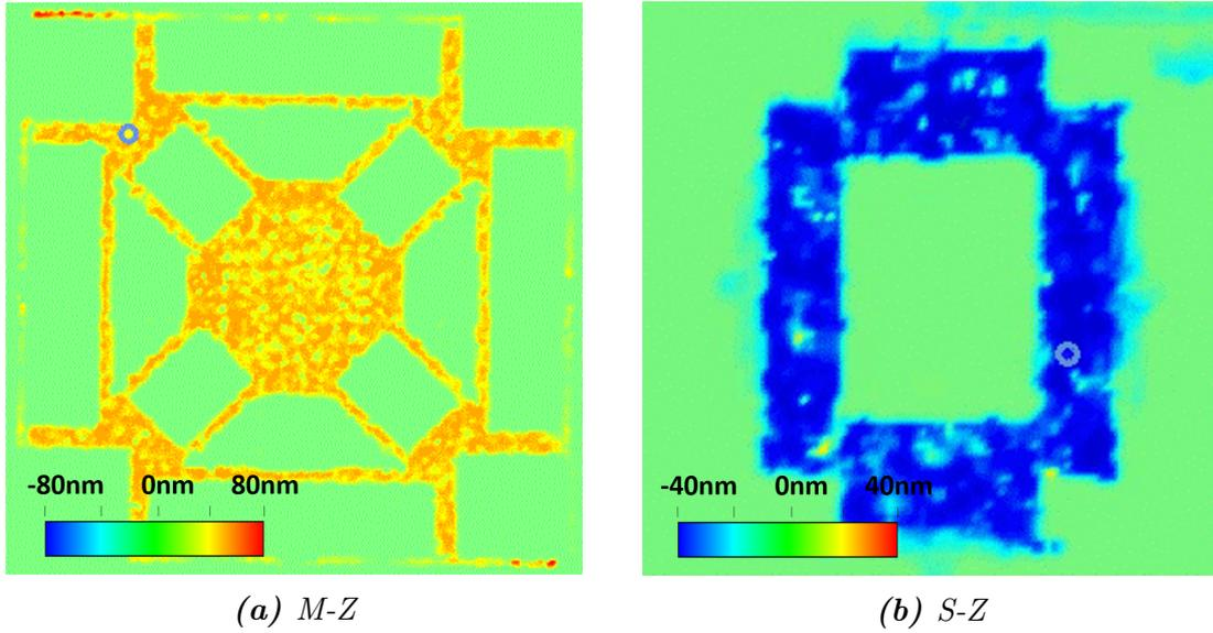
**Figure 5.7:** Doppler vibrometer measurement performed on M-Z and S-Z sensors in order to measure out-of-plane motion. The devices are actuated at resonance. The displacement of each device is represented according to the relative color scales. Both accelerometers show a pure translational movement.
