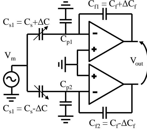
**Figure 3.6:** Schematic view of a double single ended differential charge amplifier. Potential asymmetry in both the stray capacitance and feedback path are considered.
