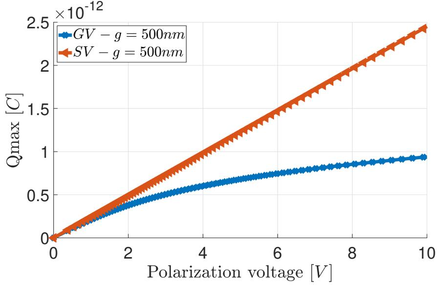
**Figure 2.13:** Delivered maximum charge versus voltage for surface variation and gap variation topologies for out-of-plane sensors assuming gap size of 500nm and parameters reported in 2.2.
