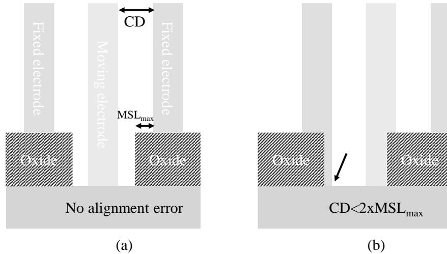
**Figure 2.4:** Two different fabrication outcome are presented: (a) Ideal situation where no misalignment is present, electrodes are centered on the oxide (b) The misalignment is larger than  $CD/2$ , some of the electrodes are partially connected to the moving layer.
