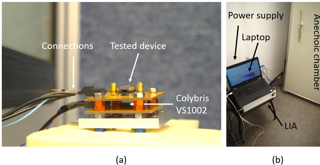
**Figure 4.11:** Images of the setup used for high-g tests: (a) the PCB hosting the device is mounted with the reference accelerometer and placed on a foam rubber base in the anechoic chamber. (b) The cables connect the PCB to the external setup: a laptop, a lock-in amplifier and a power supply.
