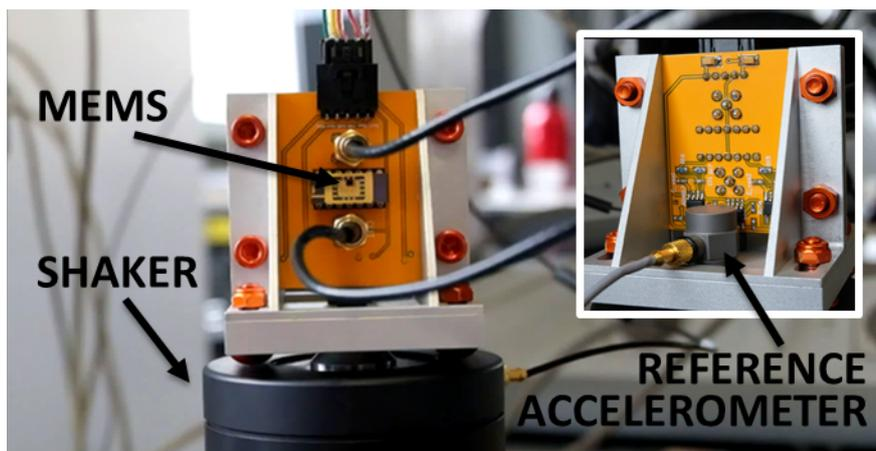
**Figure 3.10:** PCB mounted on a shaker during characterization of commercial accelerometers. One side of the PCB carries the socket and the connectors, while the electronic components are soldered on the other side.
