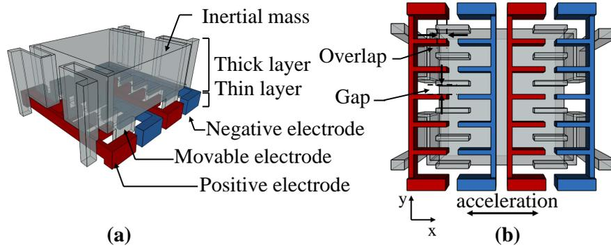
**Figure 1.7:** (a) Schematic view of the 2-layer in-plane accelerometer: mass and springs are implemented in the thick layer while electrodes are obtained from the thin one. Fixed elements are anchored to a substrate below the structure; (b) details of the comb sensing region: capacitive detection is implemented by surface variation between the fixed electrodes and the moving ones which are directly connected to the thick layer.
