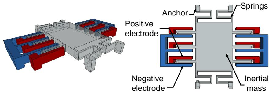
**Figure 1.3:** Schematic view of a standard in-plane capacitive accelerometer. A moving mass is suspended by springs while detection is obtained by differential capacitive variation with respect to fixed electrodes. The electrical contacts are fabricated in a poly-silicon layer deposited on the substrate. This layer is used only for electrical connection and has no mechanical use.
