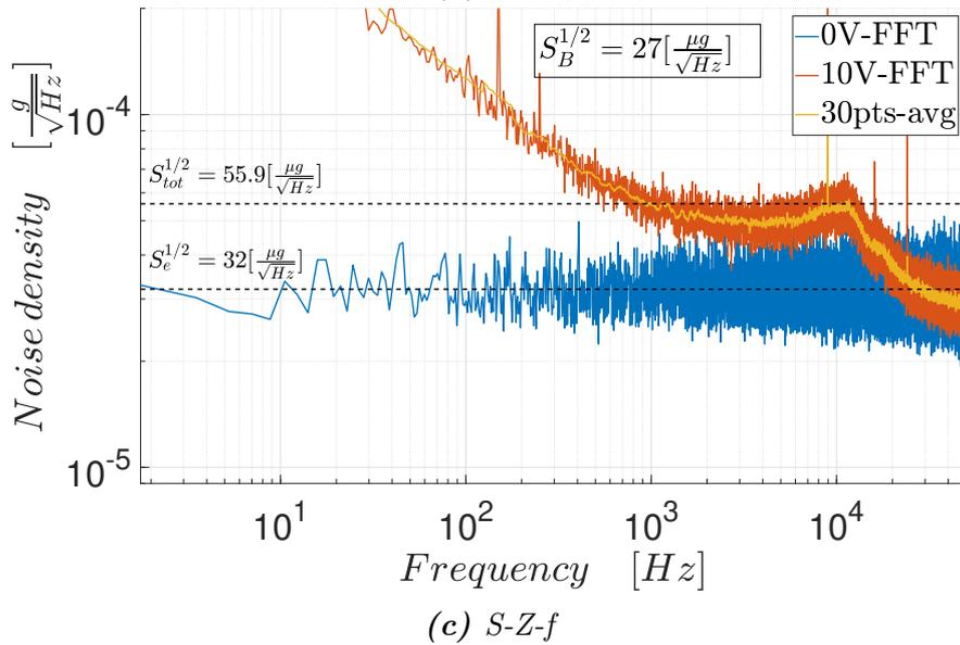
**Figure 5.9:** FFT measurement for three type of Z-devices. As for in-plane sensor the electronic noise floor is evaluated with  $V_m = 0$  while the total noise is obtained by polarizing the device  $V_m > 0$ . The device noise is extracted from the resonance peak value in order to avoid low-frequency noise contributions.
