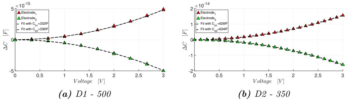
**Figure 4.6:** Examples of capacitance versus voltage measurement.
