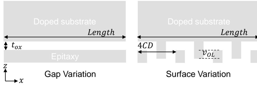
**Figure 2.12:** Schematic cross section of two possible detection methods using novel fabrication process. A single-ended view is represented for clarity, however differential detection is possible in both cases.
