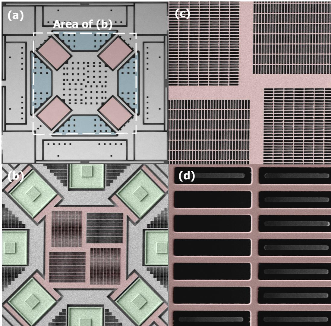
**Figure 5.3:** SEM images of the device M-Z: (a) Top view of the device at the end of the process (b) Bottom view of the device before wafer bonding, the moving mass is highlighted with a white dashed line (c) Zoom on the central electrode suspended grid (d) Image of the comb-fingers region in the suspended grid. Image is food-colored in order to highlight each element of the device: electrodes (red, jade-green), anchor points (green); mass and springs anchor points are not colored.
