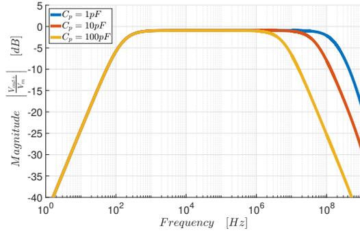
(b) Sweep of parasitic capacitance value. The value of the stray capacitor is swept from 1pF to 100pF. The gain of the circuit in the flat area is not affected, while the closed-loop pole frequency is reduced for larger value of parasitic.
