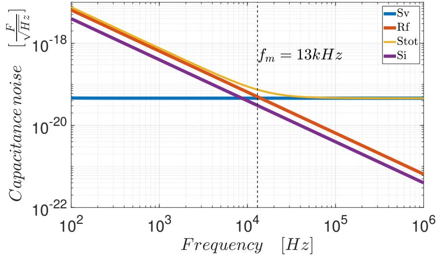
**Figure 3.4:** Input-referred noise expressed in terms of  $F/\sqrt{Hz}$  according to matlab model of the charge amplifier. The input-referred noise of the operational amplifier becomes the dominant source of noise already around 20kHz thanks to the increased feedback resistor value.
