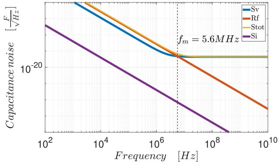
**Figure 3.3:** Numerical simulation of the three main noise sources in the trans-impedance circuit. The impact of the current sources (red, purple) decreases with frequency, while the term related to the voltage noise (blue) remains the intrinsic detection limit. In order to be voltage-noise limited, the working frequency should be higher than 5.6MHz.
