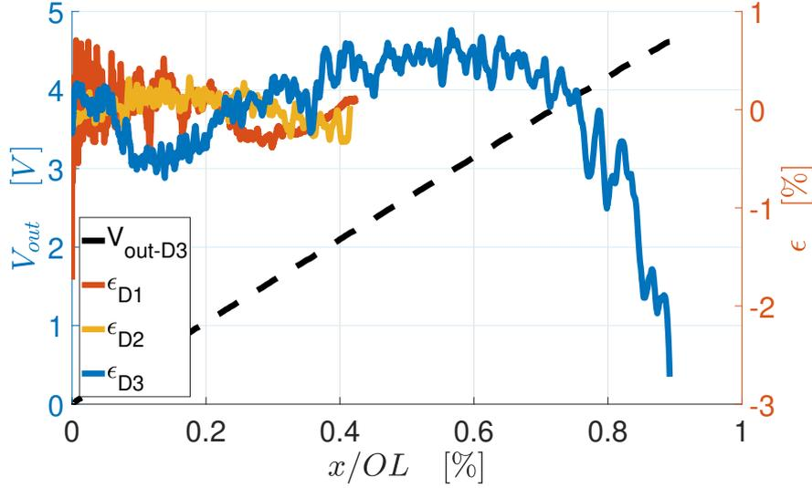
**Figure 4.10:** Rate table measurement using custom electronic and devices 1-2-3, signal modulation and demodulation is performed with a LI model SR830 from Stanford Research System: output voltage and linearity errors versus acceleration signal. The devices are polarized with 500mV signal at 100kHz, the lock-in amplifies the demodulated signal by a factor  $10/\sqrt{2}$  before acquisition. The linearity error is evaluated with respect to the linear fit of the data as a % of the FSR.
