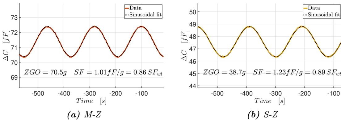
**Figure 5.8:** Scale factor and ZGO evaluation for devices M-Z and S-Z. The actuation voltage ( $V_m$ ) was set at 0.1V and 0.2V respectively. Devices were tilted at 2 dps leading to a sinusoidal acceleration of 5.5 mHz. A 4th order 200 mHz LIA filter was used to filter the signal.
