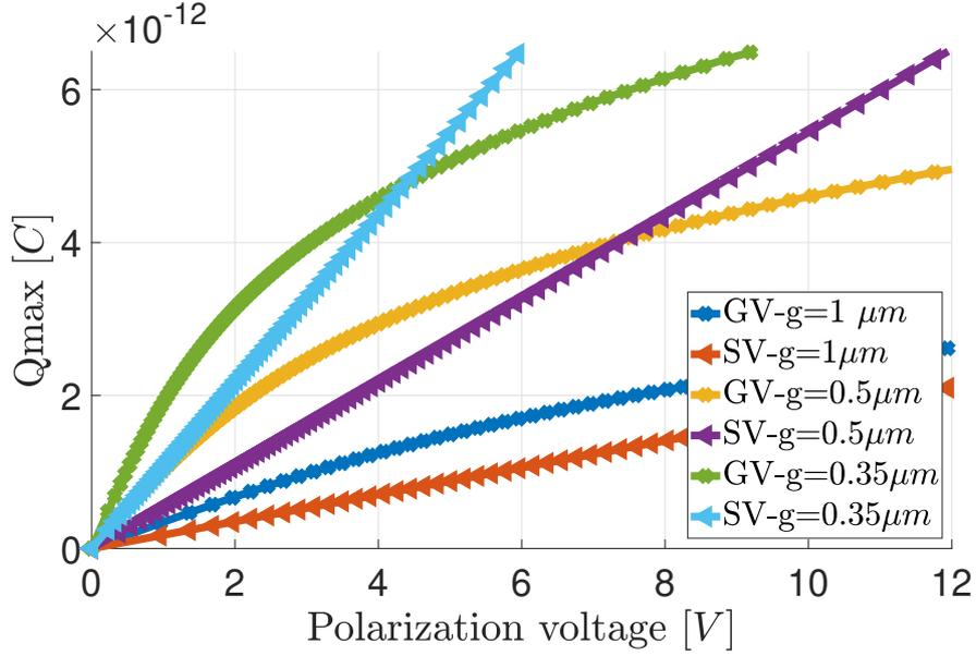
**Figure 2.10:** Delivered maximum charge versus voltage for surface variation and gap variation topologies at three different gap sizes:  $1\mu m$ ,  $0.5\mu m$  and  $0.35\mu m$ . Scaling the gap lowers the voltage at which the surface variation becomes more efficient, allowing to reach better performances also at low voltages.
