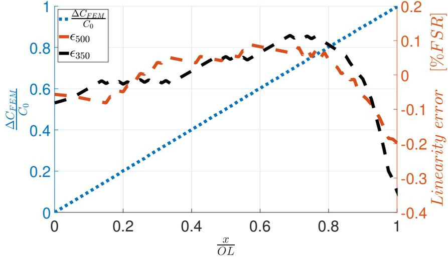
**Figure 2.15:** Plot of the relative capacitive variation and related linearity error with respect to the displacement of the moving comb normalized to the initial overlap for both 500 and 350nm devices. According to simulation the linearity remains within 1% also beyond complete static capacitance variation thanks to fringe fields and differential detection.
