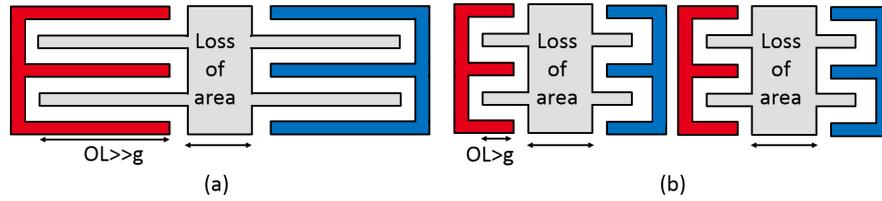
**Figure 2.9:** Possible configurations for surface variation detection: (a) large overlap allows large capacitive density, but the travel range is limited; (b) small  $OL$  allows the use of the entire linear range at the cost of reduced capacitive density.
