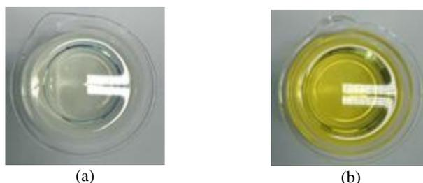
Fig 3.13 - DBT appearance: (a) new condition and (b) after measurement at 350°C
