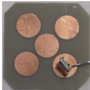
Fig. B. 1 - AlN substrate for AC and DC breakdown measurements
