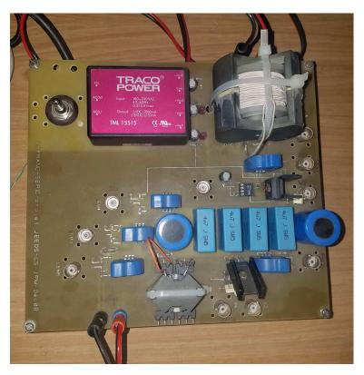
FIGURE 5.4 – SEPIC converter test bench.
