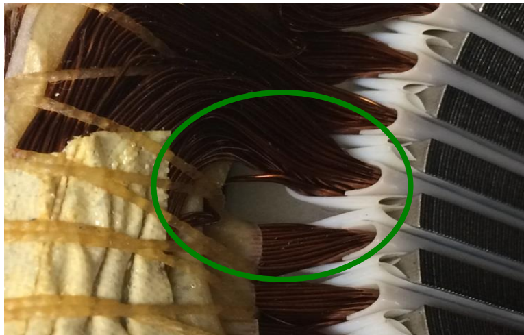
Figure 2.39. Stator winding fault in a low-voltage asynchronous motor: wire from phase V is misplaced and is in contact with a coil of phase W
