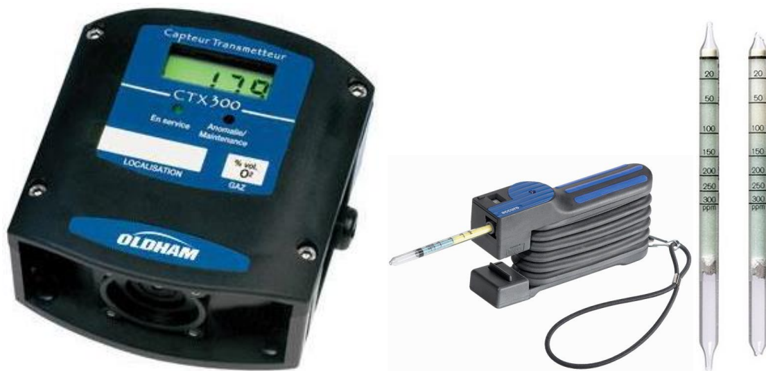
Figure 3.56. Ozone detector Oldham CTX 300 O_3 0.00 - 1.00 \pm 0.01 [ppm] (left) and 10/A Dräger Ozone Tubes 20 - 300 \pm 50 [ppm] (right) [118] [119]
