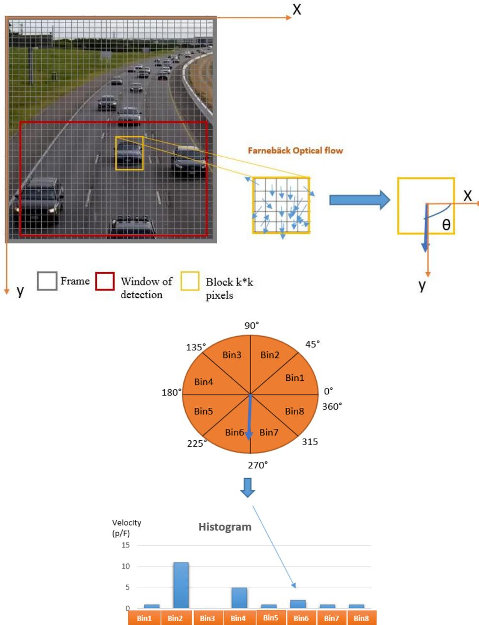
**Figure 18:** A schematic explanation of the histogram computation
