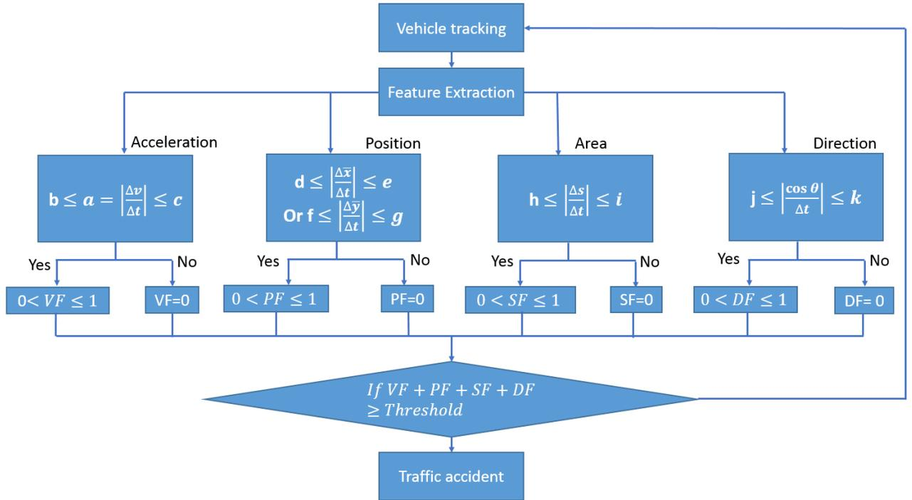
**Figure 12:** Accident detection algorithm flowchart.  $V$ ,  $(x, y)$ ,  $s$ ,  $\theta$  are respectively the velocity, the coordinate of the centroid of the vehicle, its surface and the angle formed between two motions vectors.  $a, b, c, d, e, f, g, h, i, j, k$  are thresholds.
