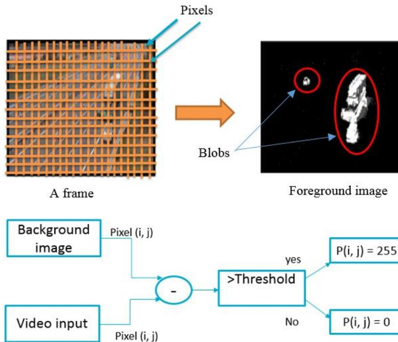
**Figure 5:** A flowchart of a basic background subtraction
