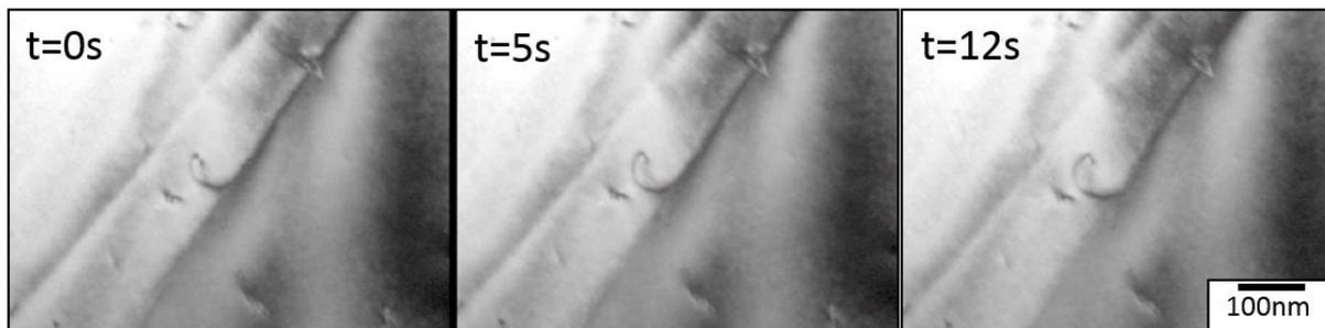
Figure 126. Dislocation loop propagation in the A3S recorded during *in situ* straining experiments.
