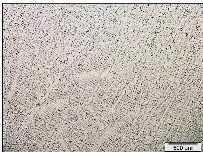
Figure 57. Optical image of the A3S in as-cast state. A dendritic structure can be seen. Dark spots are a result of etching.
