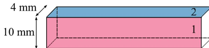
Figure 33 – Representation of the two sections analyzed by nano-indentation. 1) Measurements made on the width of the sample, 2) measurements made on the thickness of the sample.
