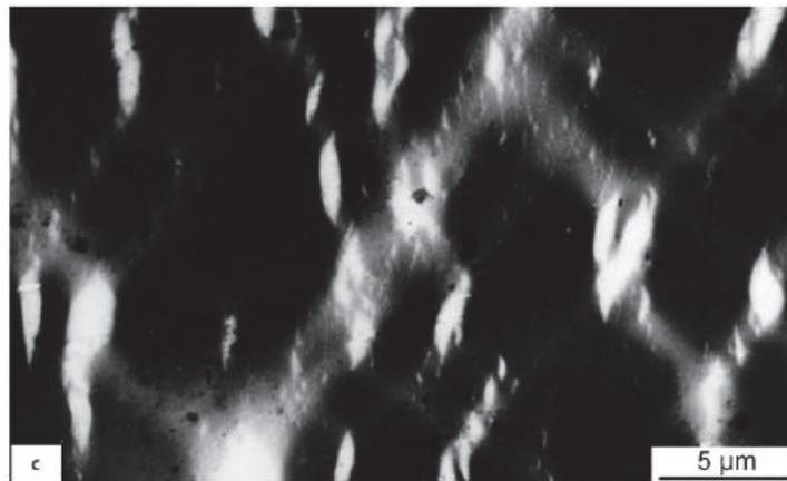
Figure 20 – Coexistence of crossed shear bands and crazes in PVC, deformed semi-thin section, deformation direction horizontal, observed by HVTEM. From [35].
