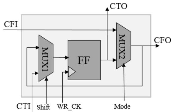
Figure 44: Wrapper-Boundary-Register (WBR) architecture
