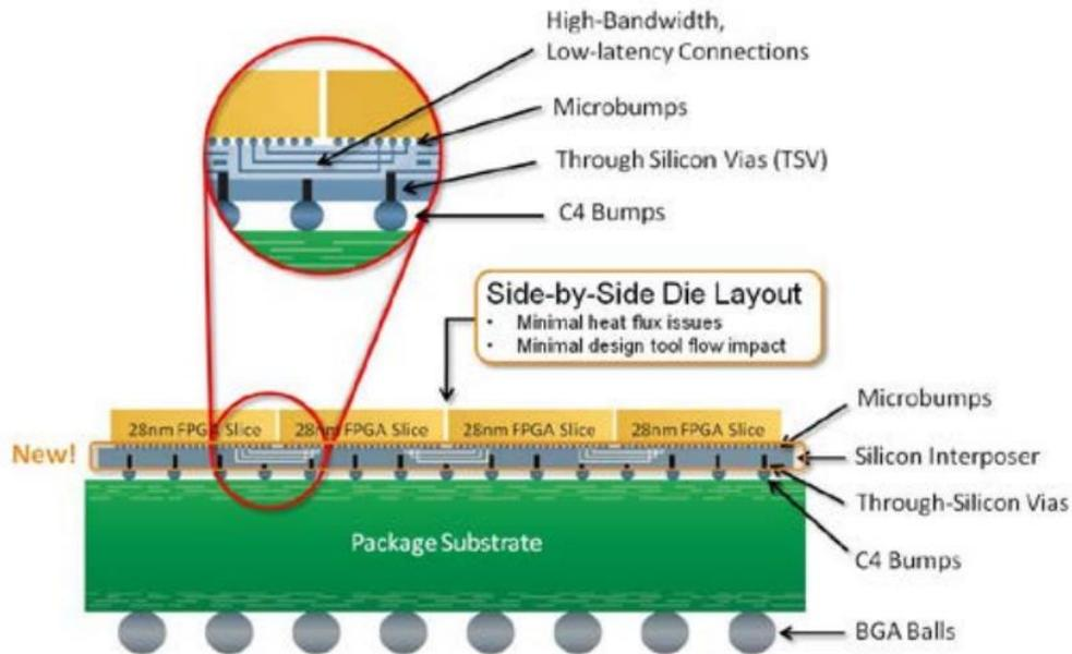
Figure 10: architecture of Virtex-7 HT (source [31])
