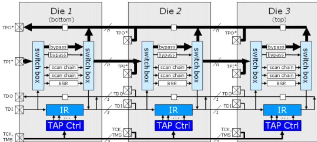
Figure 42: 3D DFT architecture based on IEEE 1149.1 (source [62])
