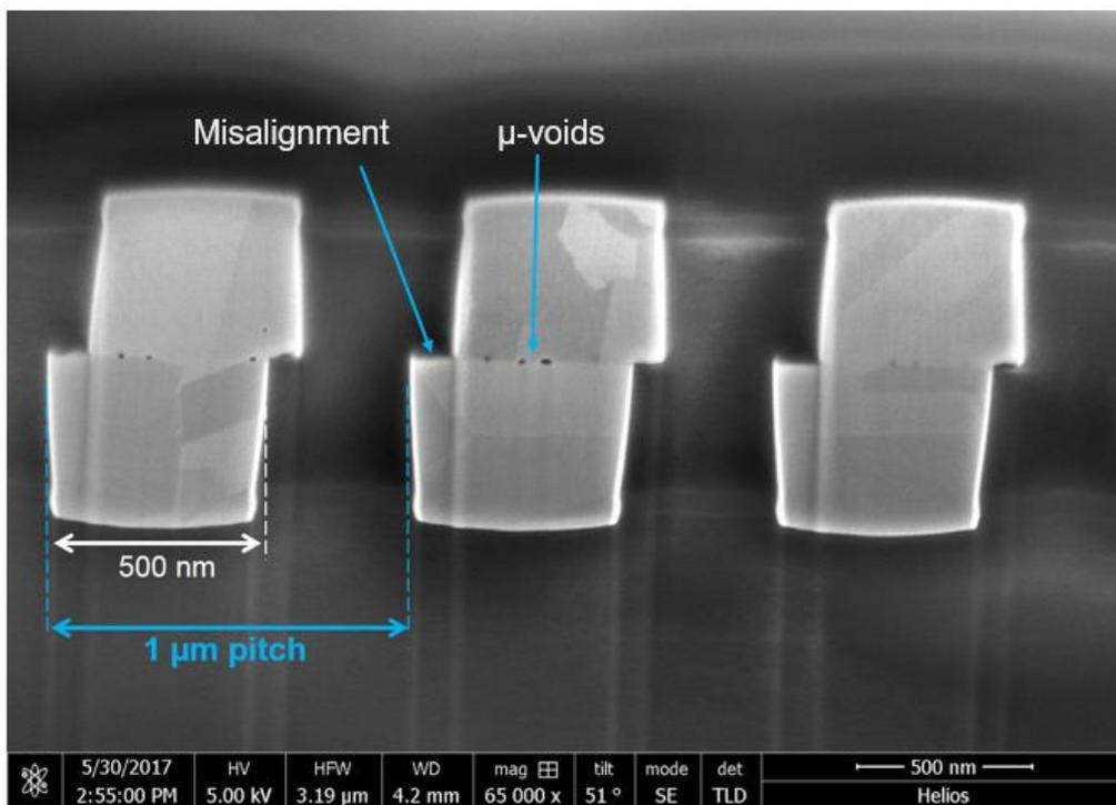
Figure 13:  $\mu$ -voids and misalignment defect in Cu-Cu interconnects
