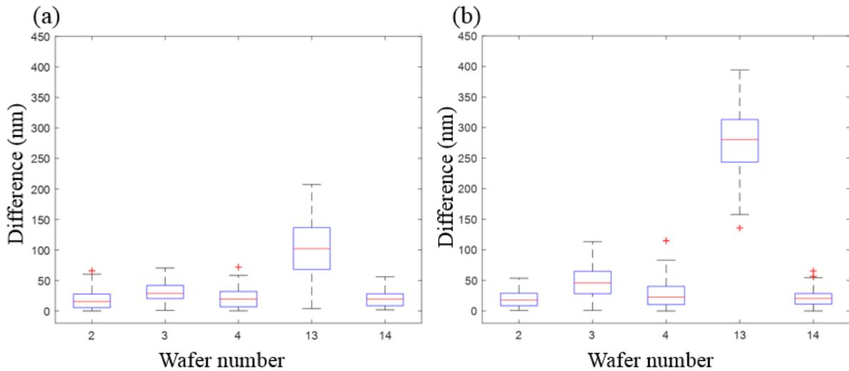
Figure 36: Comparison of test structure results ( $1.44\mu\text{m}$  pitch) and overlay measurements in X and Y direction
