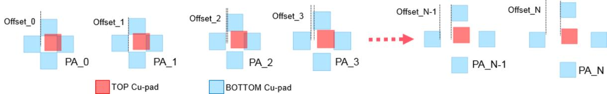
Figure 26: *N* patterns using different “offset” values
