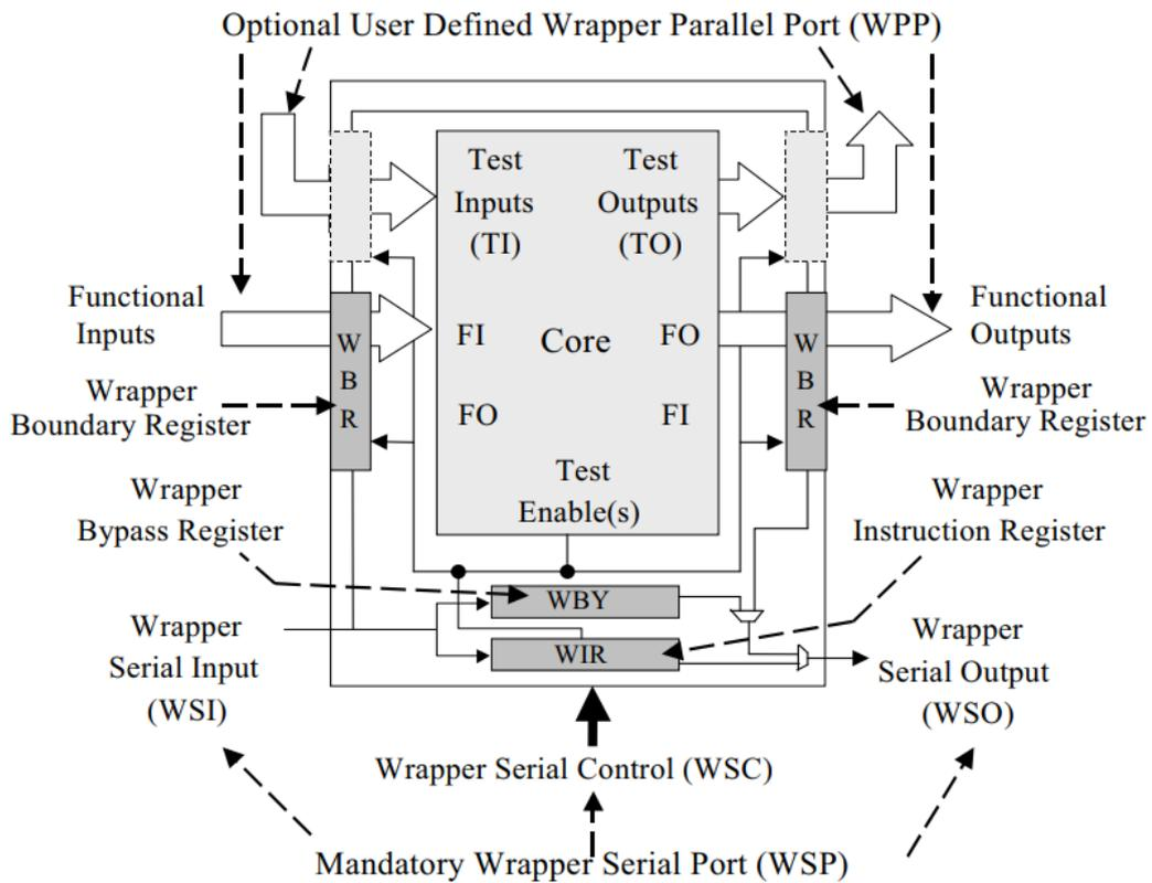
Figure 43: IEEE Std 1500 wrapper components (source [58])
