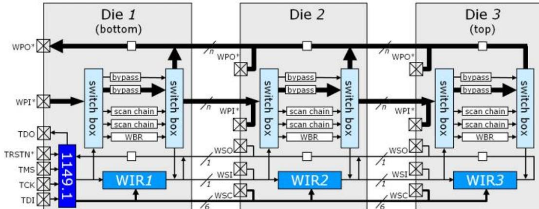
Figure 45: 3D DFT architecture based on IEEE 1500 (source [62])
