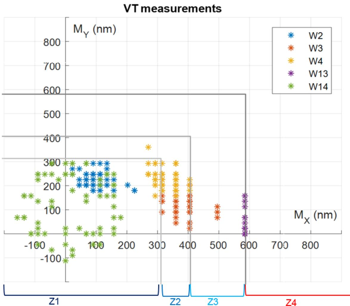
Figure 31: Misalignment test structure results (Pitch=  $1.44\mu\text{m}$ )
