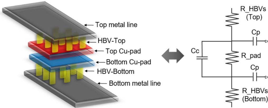
Figure 16: Equivalent electrical model of Cu-Cu interconnects
