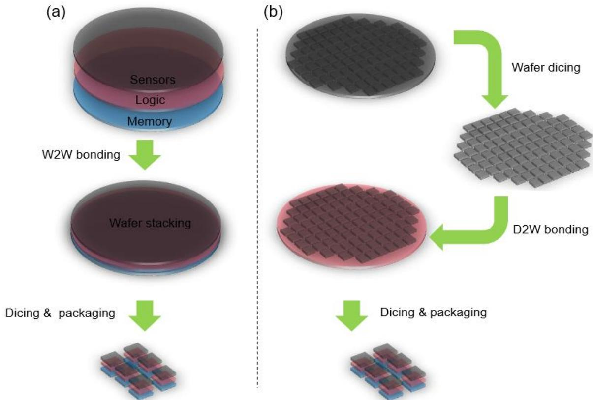
Figure 3: 3D stacking options: (a) W2W, (b) D2W
