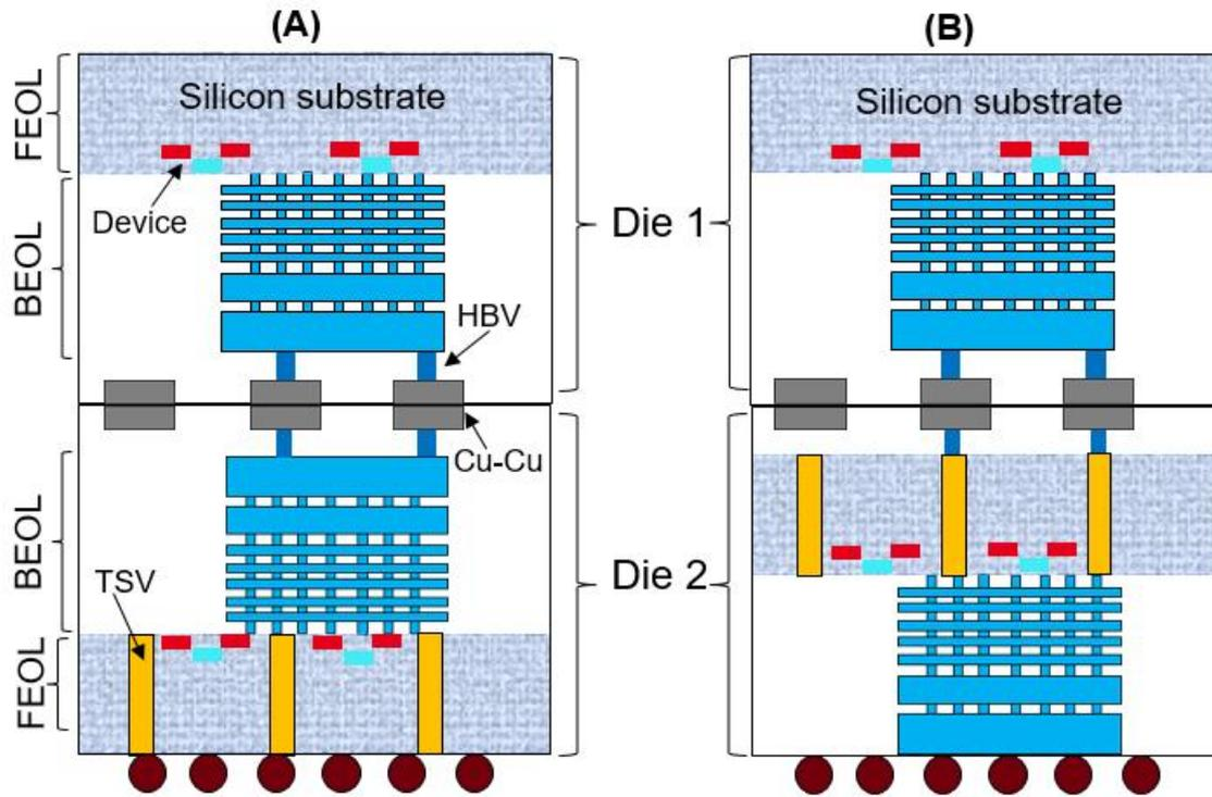
Figure 5: Cross-sectional view of high density 3D-IC structures:
