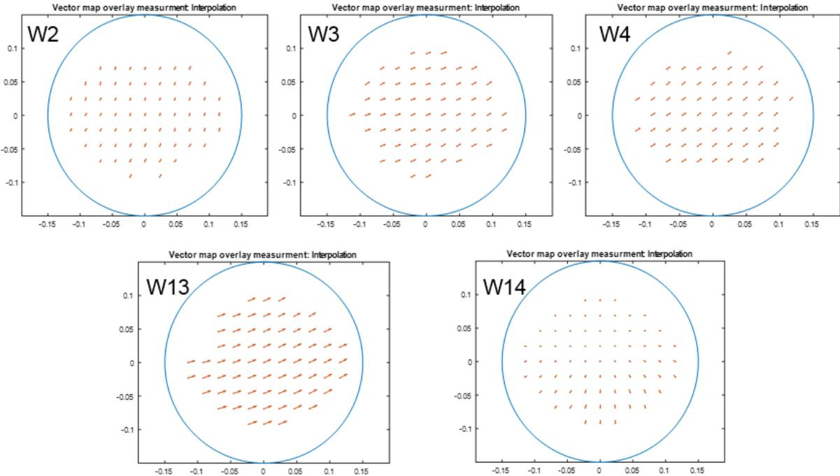
Figure 34: Wafer map results using overlay measurements
