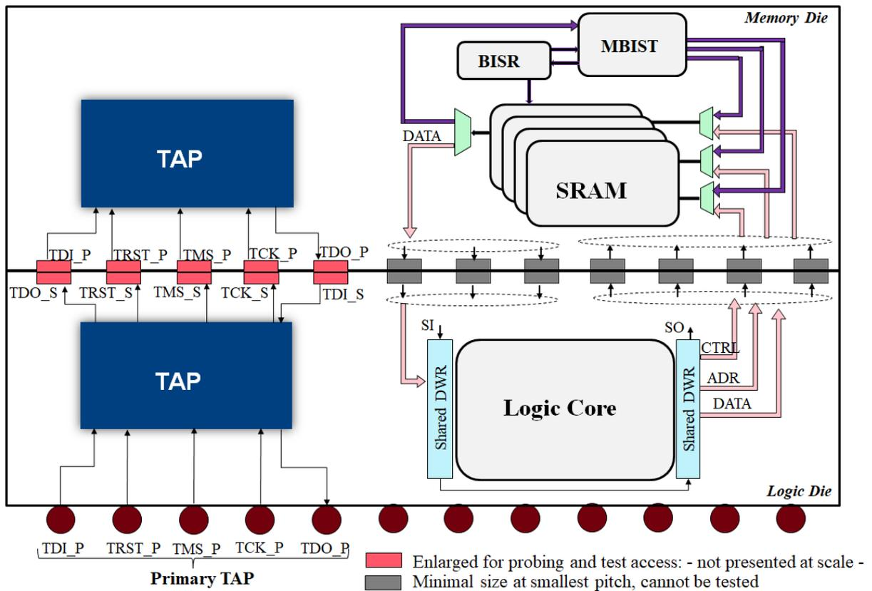
Figure 53: Optimized DFT architecture for SRAM/Logic 3D-IC
