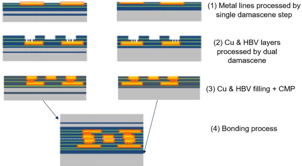
Figure 6: Example of hybrid bonding process flow (source [15])
