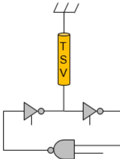
Figure 56: Test TSV using ring oscillator example
