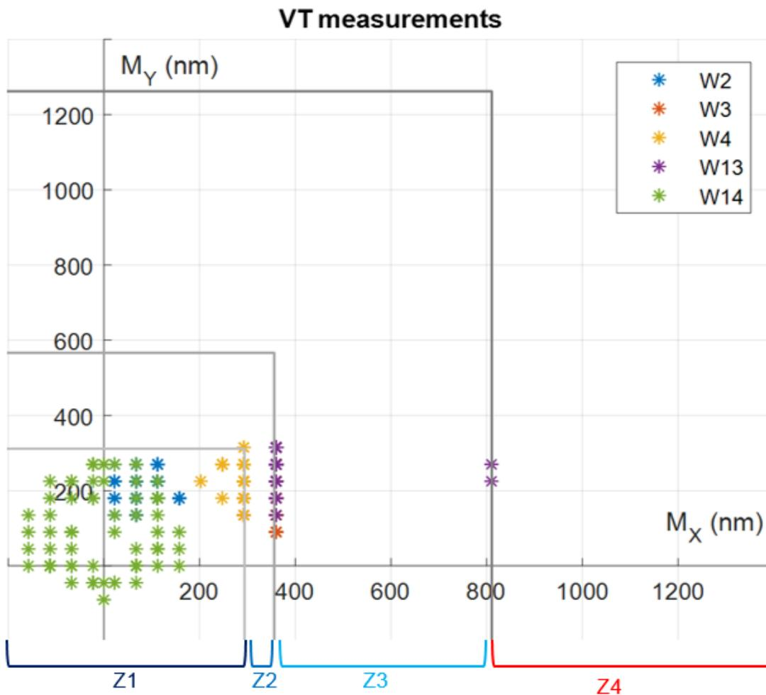
Figure 29: Misalignment test structure results (Pitch=  $3.42\mu\text{m}$ )
