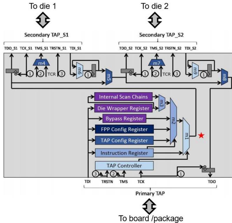
Figure 48: Serial control mechanism (SCM) (source: [68])
