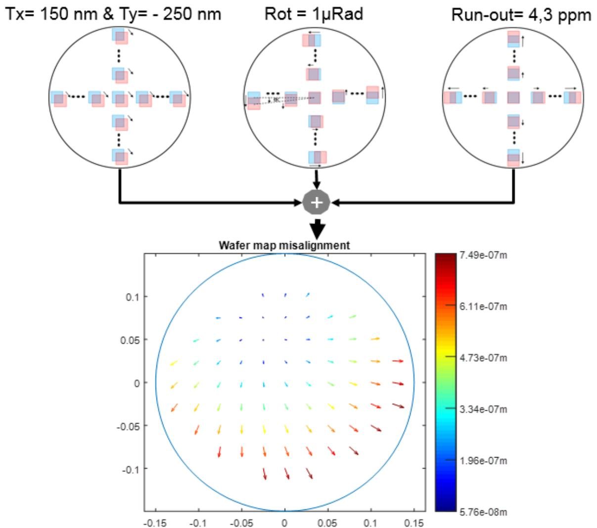
Figure 24: Wafer map: example of misalignment simulation
