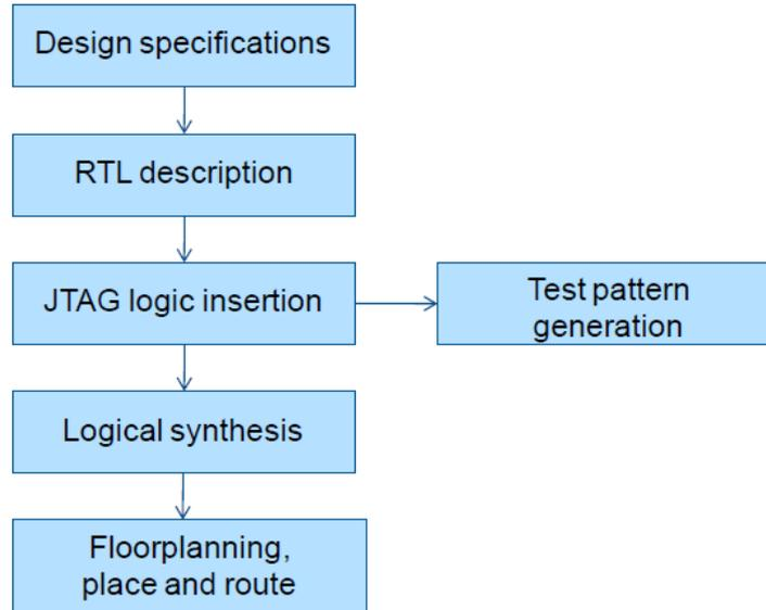
Figure 65: Design flow of the test chip circuit
