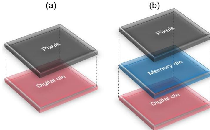
Figure 8: Structure of stacked CMOS image sensor:
