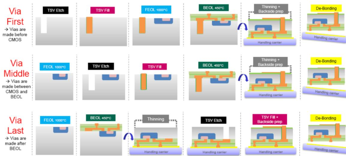
Figure 7: Via-first, via-middle and via-last illustration (source [16])
