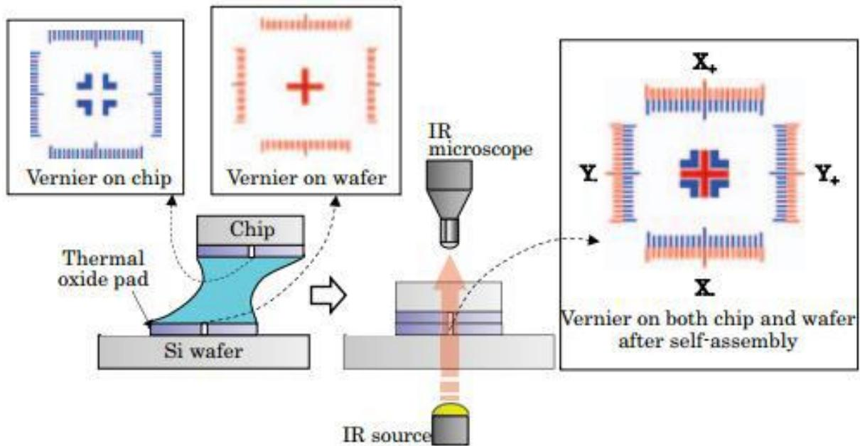
Figure 21: IR metrology tool principle (source [50])
