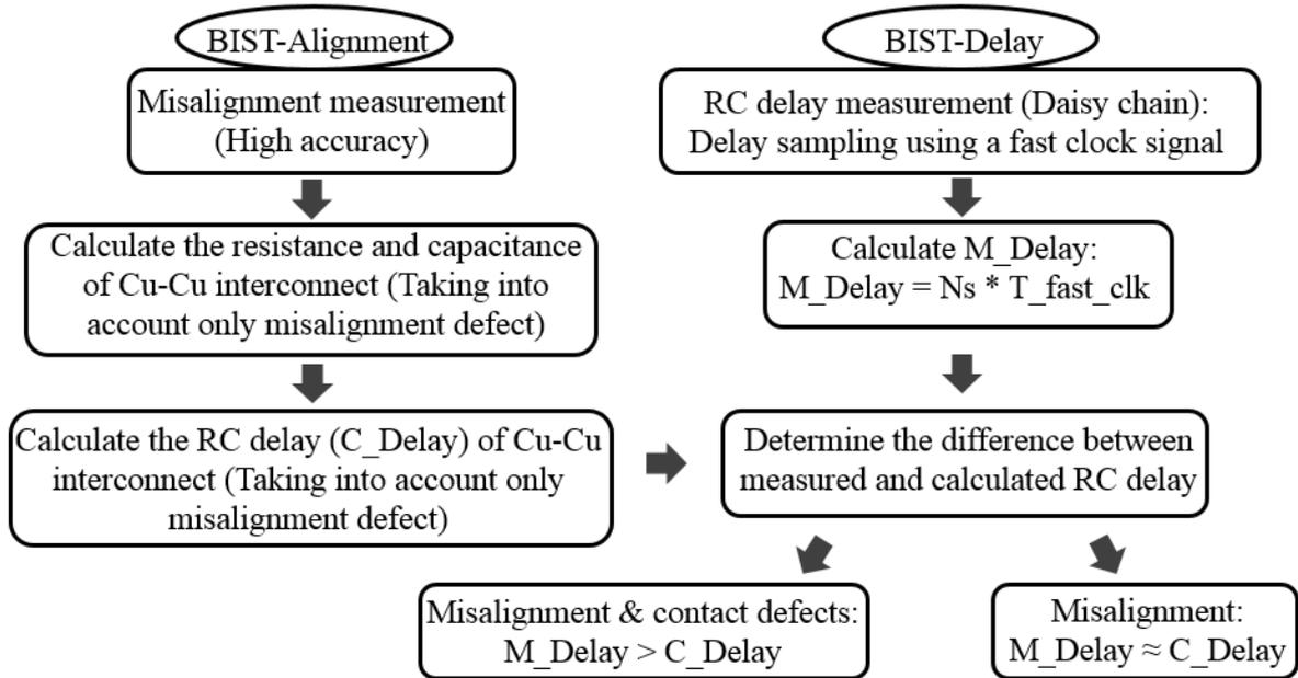
Figure 57: Proposed structural test flow for Cu-Cu interconnects
