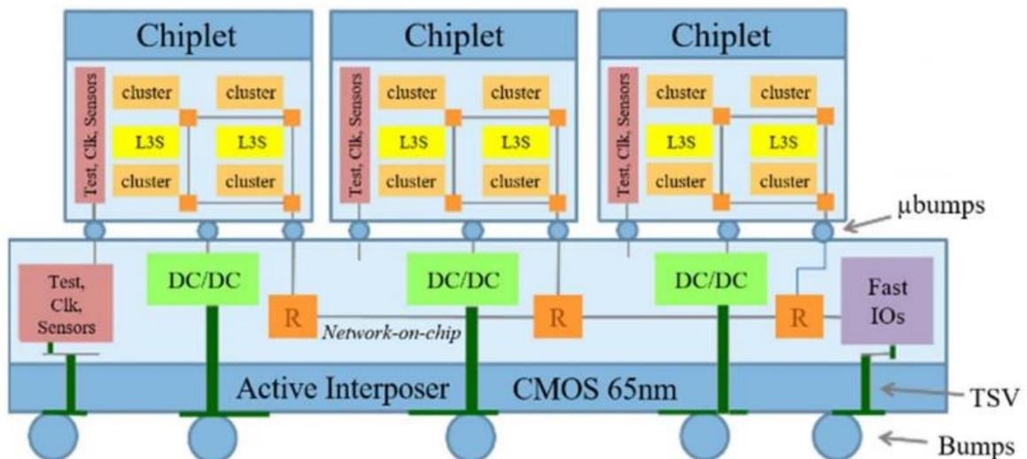
Figure 12: Intact system architecture overview (source [38])
