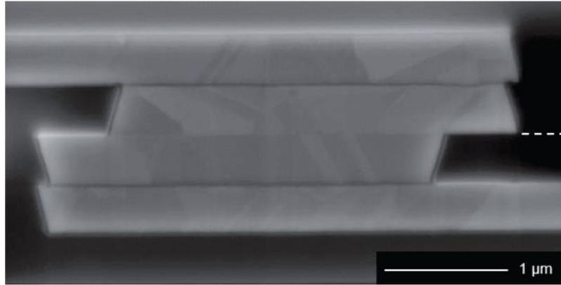
Figure 22: Example of SEM image of Cu-Cu interconnect (source [55])
