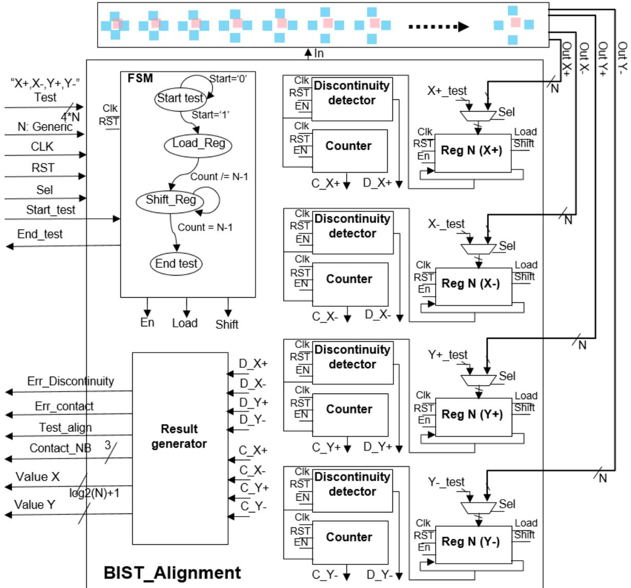
Figure 58: Proposed structural test flow for Cu-Cu interconnects
