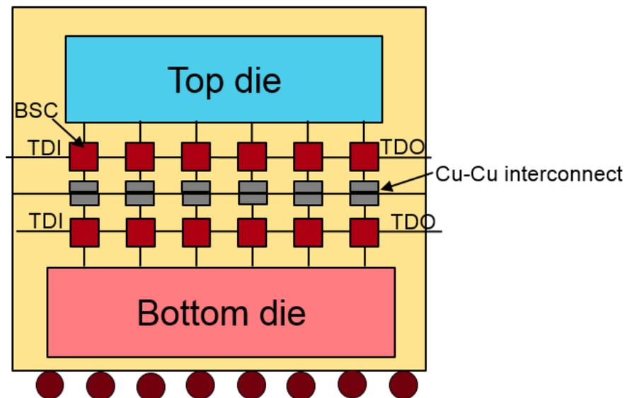
Figure 15: Test of 3D-IC interconnects at system level
