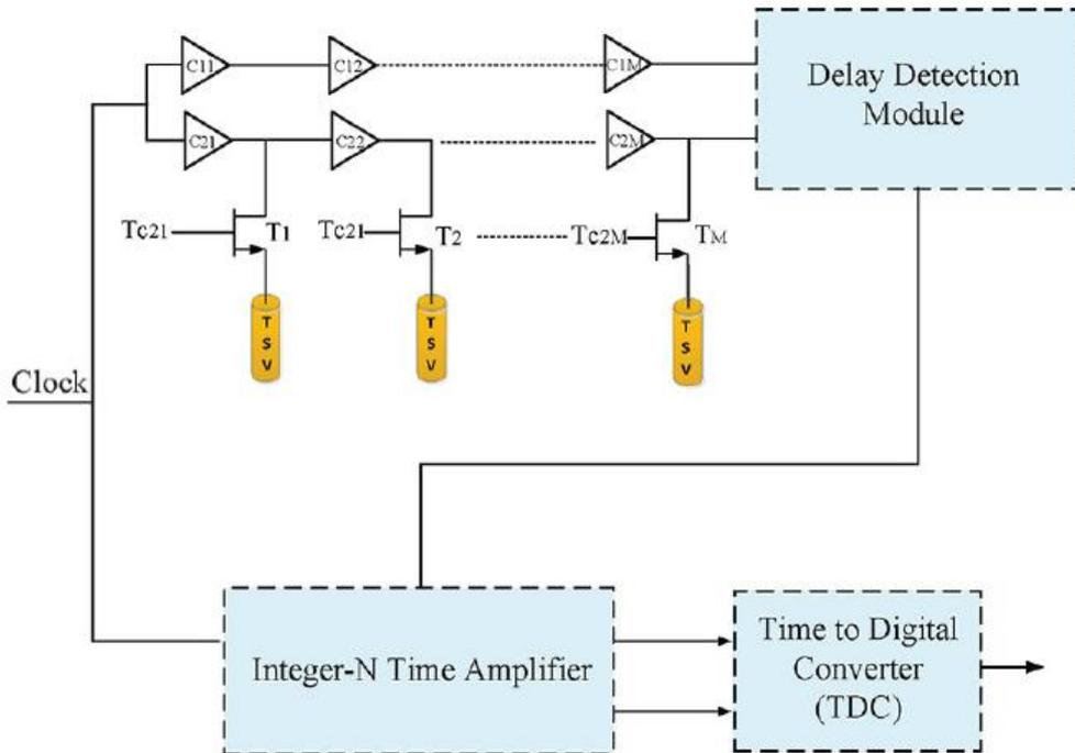
Figure 55: Example of delay measurement method (source [71])
