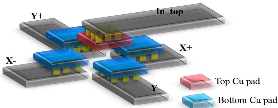
*Figure 25: The reference pattern of misalignment test structure*
