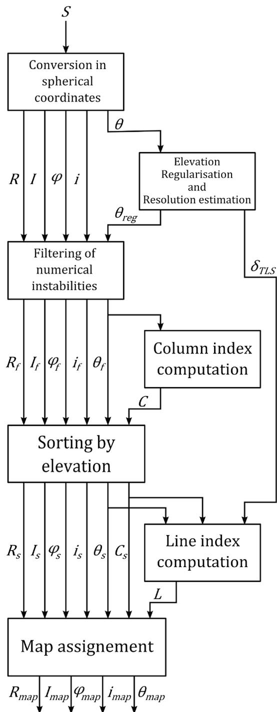
Figure 4.3 – General principle of the equirectangular projection algorithm
