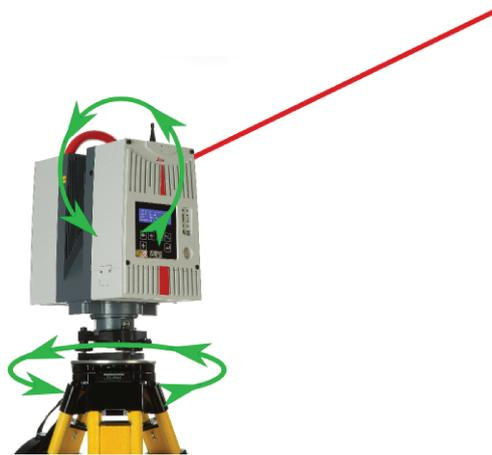
Figure 2.2 – TLS sampling principle, in green the rotation of the azimuthal and zenithal motors
