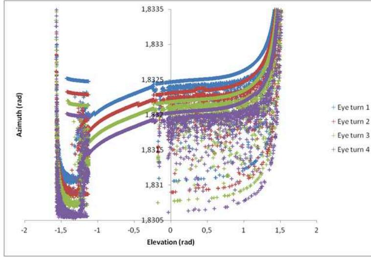
Figure 4.2 – Recorded azimuth versus recorded elevation for a scan in ultra resolution ( $\frac{\pi}{4}10^{-4}$ ). In blue green red and purple are the values of azimuth versus elevation for four consecutive scanner eye turns (each color corresponds to the points acquired during a specific turn)
