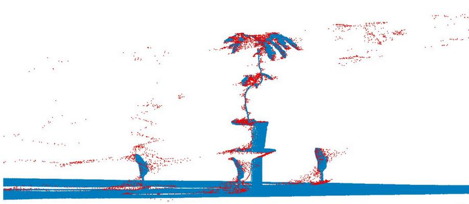
Figure 1.4 – Example of mixed point noise, in blue the valid points, in red the mixed points
