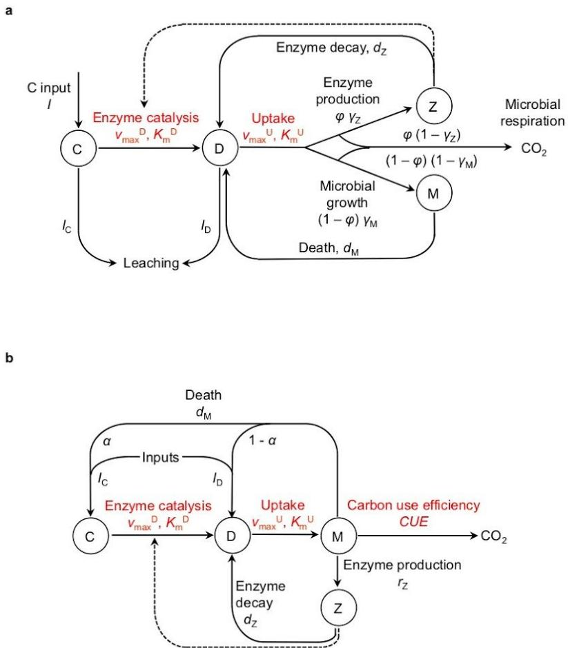
**Extended Data Figure 1 | Structure of soil microbial decomposition models.** **a**, Our model assumes dynamic allocation of assimilated carbon to enzyme production, whereas in **b**, Allison *et al.* (2010)'s model<sup>11</sup>, enzymes are produced at a constant rate.
