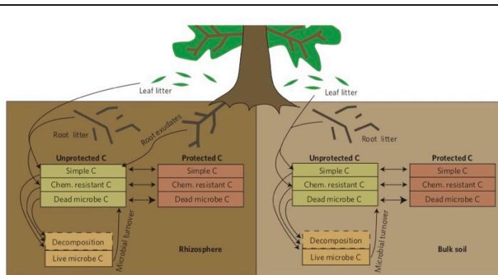
**Figure 4. Structure of Sulman *et al.* (2014)'s model.** Soil carbon is divided into three chemical classes, which can be protected or unprotected. Decomposition is mediated by microbial biomass, which takes up a portion of decomposed carbon and loses carbon to CO<sub>2</sub> and the dead microbial C pool over time. Soil is separated into the rhizosphere, which receives root exudate inputs, and bulk soil, which does not. (Reproduced from Sulman *et al.* 2014)
