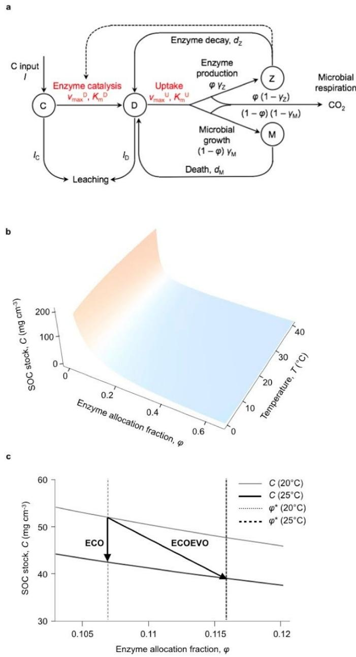
**Figure 1. Effect of temperature and enzyme allocation fraction on SOC ecological equilibrium.** **a**, Structure of the microbial-enzyme ecological model (see Methods for details): SOC stock is the balance of plant input,  $I$ , and loss by exoenzyme-mediated degradation to DOC ( $D$ ), which in turn is allocated between (fraction  $\varphi$ ) production of
