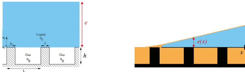
FIG. 1. (Color online) Sketch of the liquid interface at a superhydrophobic wall in the Cassie state.  $L, h$ : roughness periodicity and height;  $a$ : typical length scale for solid/liquid contact areas.
