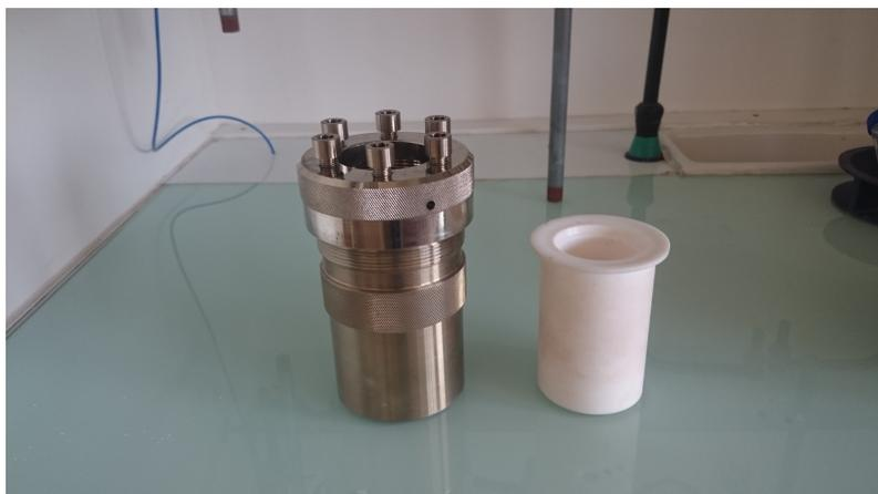
Figure 3.2: Teflon beaker and pressure reactor used for the  $\text{CuFeO}_2$  nanoplatelet synthesis.
