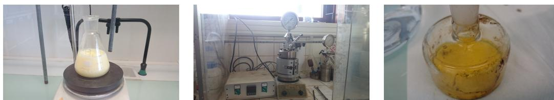
Figure 3.1:  $\text{BiVO}_4$  synthesis: left: foaming aqueous mixture of bismuth precursor, vanadium precursor and sodium dodecyl sulphate (SDS); middle: treatment in pressure reactor; right: yellow  $\text{BiVO}_4$  precipitate after removal from pressure reactor.
