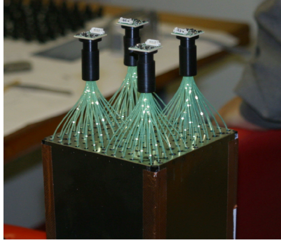
Figure 4.7: Prototype EMCal module where the back enclosing structure has been removed in order to show the fibres bundled into the APDs.
