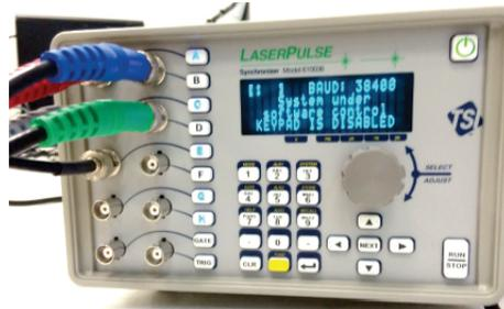
Figure 30: The LASERPULSE synchronizer
