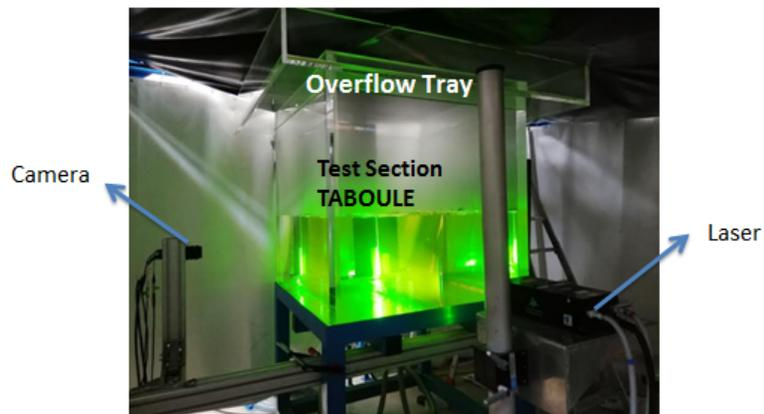
Figure 59: Test section TABOULE
