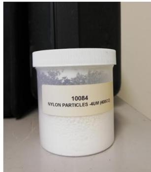
Figure 32: PIV Particles
