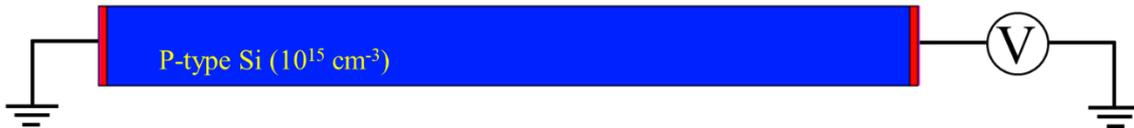
Figure III.17: Structure used to study metal-semiconductor contacts.
